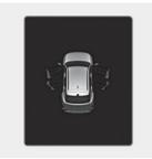
This warning appears if any door or hood or liftgate is left open. The warning indicates which door is open on the cluster display.
