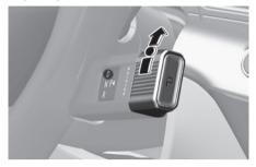
To shift the gear to D (Drive), rotate the rotary shifter to D (Drive) while depressing the brake pedal.
