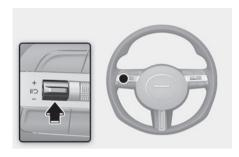
Press the **II 2** switch to temporarily pause the set speed limit. The set speed limit will turn off but the Speed Limit (**STLIMIT**) indicator will stay on.
