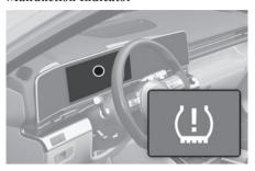
The TPMS Malfunction Indicator (<u>U</u>) illuminates after it blinks for about one minute when there is a problem with the Tire Pressure Monitoring System.
