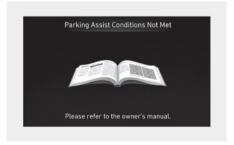
When "Parking Assist Conditions Not Met" message appears when Parking/View (P) button has been pressed and held while Remote Smart Parking Assist is in standby. After a while, press and hold the Parking/View (P) button again to see if Remote Smart Parking Assist works.
