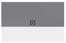
The gear shift indicator indicates the current rotary shifter position (D, N, R) or P (Park).
