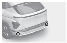
[A] Rear corner radar Refer to the picture above for the detailed location of the detecting sensors.
