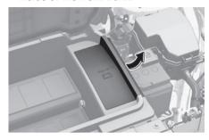
6. Remove the motor compartment fuse box cover.
