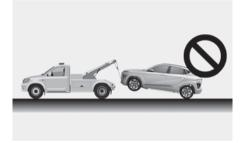
• Do not lift using the trailer hitch or body and chassis part.
