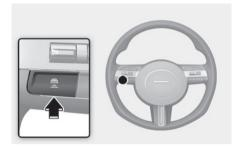
Press the button repeatedly to cycle through the headway settings from Distance  $4 \rightarrow$  Distance  $3 \rightarrow$  Distance  $2 \rightarrow$  Distance  $1 \rightarrow$  Distance  $4 \rightarrow$
