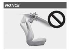
If you adjust the seatback towards the front with the head restraint and seat cushion raised, the head restraint may come in contact with the sunvisor or other parts of the vehicle.
