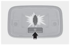
ᅜ: Press the button to turn on and off the rear room lamp.
