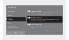
With the Start/Stop button in the ON position, press the SETUP button, and then select Vehicle > Lights > High Beam Assist to turn on High Beam Assist and deselect to turn off the function.
