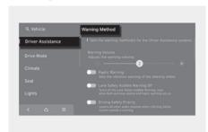
With the vehicle on, press the SETUP button, and then select **Vehicle > Driver Assistance > Warning Methods** in the infotainment system to select following:
