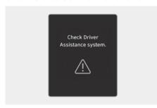
When Smart Cruise Control is not working properly, the "Check Driver Assistance system." warning message will appear, and the "\( \tilde{\Delta}\)" warning light will illuminate on the instrument cluster. Have your vehicle inspected by an authorized HYUNDAI dealer.
