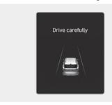
Brake control will end after the vehicle is stopped by emergency braking for about 2 seconds.
