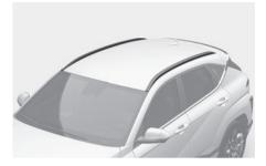
Your vehicle may come equipped with roof side rails. If your vehicle is equipped with roof rack rails, you can add roof rack crossbars as an accessory (not shown).
