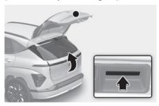
When the liftgate is closed, press the power liftgate open/close button to open the liftgate.
