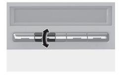
Push up the switch to increase fan speed and airflow. Push down the switch to decrease fan speed and airflow.
