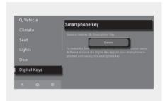
To delete only my registered digital key (smartphone), press the SETUP button, and then select Vehicle > Digital Keys > Smartphone key > My Smartphone Key > Delete in the infotainment system.
