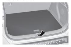
Remove the top board and insert the top board all the way in along the lower groove on both sides.
