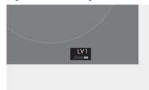
The selected regenerative braking level appears on the instrument cluster.
