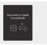
In traffic, your vehicle will stop if the vehicle ahead of you stops. Also, if the vehicle ahead of you starts moving, your vehicle will start as well. In addition, after the vehicle has stopped and a certain time have passed, the "Use switch or pedal to accelerate" message will appear on the instrument cluster. Depress the accelerator pedal or operate the + switch, - switch or IIO switch to start driving.
