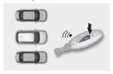
Press and hold the Remote Start button ( ) within 4 seconds until the vehicle starts.
