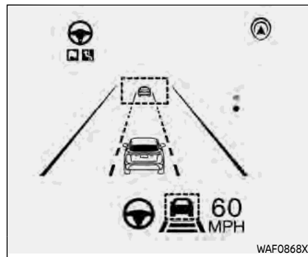
System set display — a vehicle detected ahead (for ProPILOT Assist 2.0)
