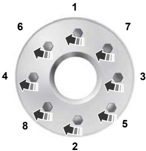
8-wheel nut torque sequence
