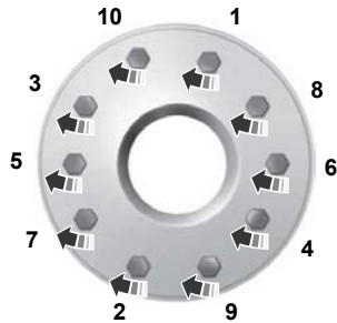
10-wheel nut torque sequence
