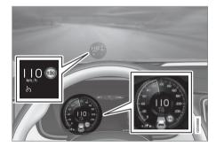
The previous illustration shows that Adaptive Cruise Control is set to maintain a speed of 110 km/h (68 mph) and that there is no target vehicle ahead to follow.
