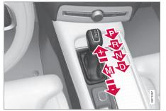
Large gear selector and gear selector positions overview.
