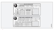
3 Tire inflation pressures. This label indicates the correct inflation pressures for the tires that were on the vehicle when it left the factory.
