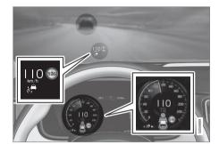
The previous illustration shows that Adaptive Cruise Control is set to maintain a speed of 110 km/h (68 mph) and is following a target vehicle ahead, which is traveling at the same speed.
