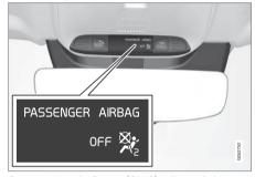
Occupant Weight Sensor (OWS) indicator light
