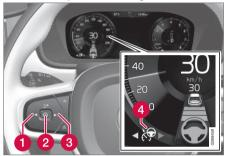
A green steering wheel indicates that Pilot Assist is providing steering assistance.
