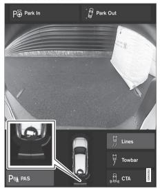
The screen can display colored sensor fields on the vehicle symbol.
