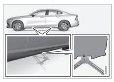
5. Position the jack under the attachment point being used, ensuring that the surface is firm, flat and not slippery.
