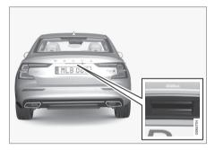
The trunk lid is held closed by an electronic locking mechanism.
