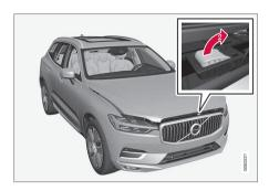
Swipe your hand from left to right under the hood, grasp the handle and move it up and to the side to release the catch and lift the hood.
