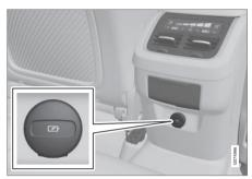
USB ports (type C) on rear of tunnel console for charging phones, tablets, etc.<sup>7</sup>.
