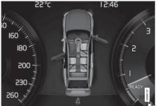
Graphics in the instrument panel with various types of warnings. The warning colors for the doors/trunk lid vary depending on the vehicle's speed.
