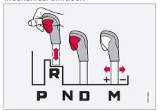
Shiftlock for vehicles with large gear selectors.
