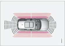
The warning signal will begin pulsating rapidly when the obstacle is less than approx. 25 cm (0.8 ft) from the vehicle.
