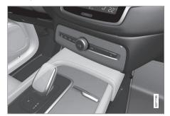
Overview of small gear selector, where it is not possible to deactivate the shiftlock.
