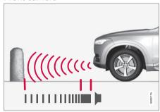
The warning signal has a continuous tone when the obstacle is less than approx. 30 cm (1 ft) from the vehicle.
