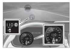
The previous illustration shows that Pilot Assist is set to maintain a speed of 110 km/h (68 mph) and is following a target vehicle ahead that is traveling at the same speed.
