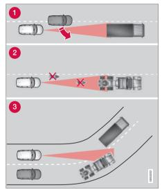
The radar sensor's field of vision
