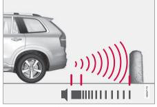
The warning signal has a continuous tone when the obstacle is less than approx. 30 cm (1 ft) from the vehicle.
