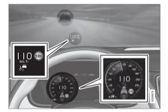
The previous illustration shows that Pilot Assist is set to maintain a speed of 110 km/h (68 mph) and is following a target vehicle ahead that is traveling at the same speed.
