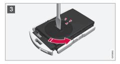
3 Use a screwdriver or similar object to turn the battery cover counterclockwise so the markers point to **OPEN**.
