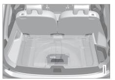
If the vehicle is instead equipped with a 48 V support battery, it is located under the cargo compartment. The box over the 48 V support battery may only be removed by an authorized workshop.
