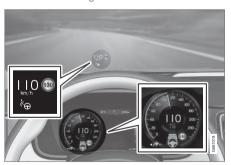
The previous illustration shows that Pilot Assist is set to maintain a speed of 110 km/h (68 mph) and that there is no target vehicle ahead to follow.
