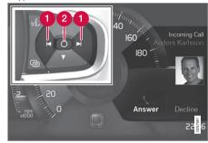
Examples of messages in the instrument panel<sup>4</sup> and the right-side steering wheel keypad.
