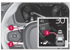
Controls for setting a time interval.
