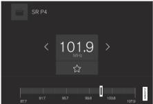
Searching manually makes it possible to find and tune to stations that are not on the automatically compiled list of the strongest stations in the area.
