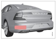
Keep the marked area clean (on both the left and right sides of the vehicle)<sup>91</sup>.
