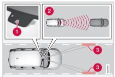
The camera/radar sensor monitors the distance to the vehicle ahead and detects lane markings.
