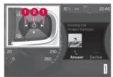
Examples of messages in the instrument panel<sup>5</sup> and the right-side steering wheel keypad. The illustration is generic - details may vary according to vehicle model.
