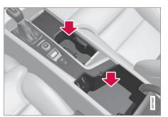
Storage compartments with cup holders, electrical outlets, wireless phone charger\* and USB ports in the tunnel console.
