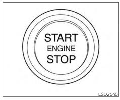
When the ignition switch is pushed without depressing the brake pedal, the ignition switch will illuminate
