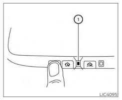
2. Using both hands, simultaneously press and hold the desired HomeLink® button and hand-held transmitter button DO NOT release until the HomeLink® indicator light (1) flashes slowly and then rapidly. When the indicator light flashes rapidly, both buttons may be released. (The rapid flashing indicates successful programming.)
