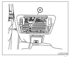
3. Remove the fuse with the fuse puller (B).
