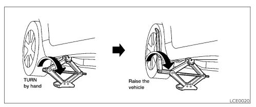
3. To lift the vehicle, securely hold the jack lever and rod with both hands. Carefully raise the vehicle until the tire clears the ground. Remove the wheel nuts, and then remove the tire.
