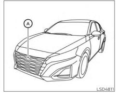
The I-FCW system uses a radar sensor (A) located on the front of the vehicle to measure the distance to the vehicle ahead in the same lane.
