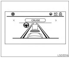
System set display with no vehicle detected ahead No vehicle detected ahead
