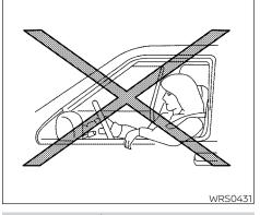
Even with the NISSAN Advanced Air Bag System, never install a rearfacing child restraint in the front seat. An inflating front air bag could seriously injure or kill your child. For additional information, see "Child restraints" (P. 1-22).
