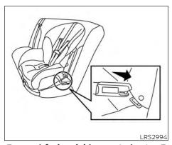
Forward-facing rigid-mounted - step 3 Do not install child restraints that require the use of a top tether strap in seating positions that do not have a top tether anchor.
