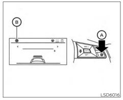
1. Push the ProPILOT Assist switch (a). This turns on the ProPILOT Assist system.
