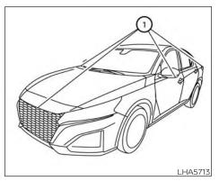
If dirt, rain or snow accumulates on any of the cameras (1), the Intelligent Around View® Monitor may not display objects clearly. Clean the camera by wiping with a cloth dampened with a diluted mild cleaning agent and then wiping with a dry cloth.
