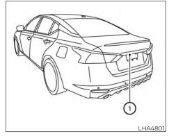
To display the rear view, the Rear View Monitor system uses a camera located just above the vehicle's license plate  $\Omega$ .
