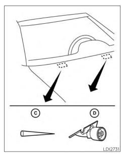
If you wax the surface of the hood, be careful not to let wax get into the washer nozzle (a). This may cause clogging or improper windshield-washer operation. If wax gets into the nozzle, remove it with a needle or small pin (3).
