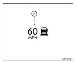
When passing another vehicle, the set speed indicator (A) flashes when the vehicle speed exceeds the set speed. The vehicle ahead detection indicator turns off when the area ahead of the vehicle is open. When the pedal is released, the vehicle returns to the previously set speed. Even though your vehicle speed is set in the ICC system, you can depress the accelerator pedal when it is necessary to accelerate vour vehicle rapidly.
