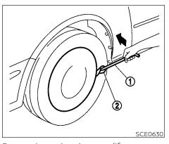
Removing wheel cover (if so equipped)
