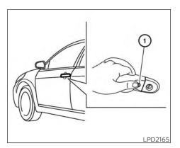
If a door handle is pulled while unlocking the doors, that door may not be unlocked. Returning the door handle to its original position will unlock the door. If the door does not unlock after returning the door handle, push the door handle request switch (if so equipped) to unlock the door.
