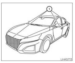
If dirt, rain or snow accumulates on any of the cameras (1), the MOD system may not operate properly. Clean the camera by wiping with a cloth dampened with a diluted mild cleaning agent and then wiping with a drv cloth.
