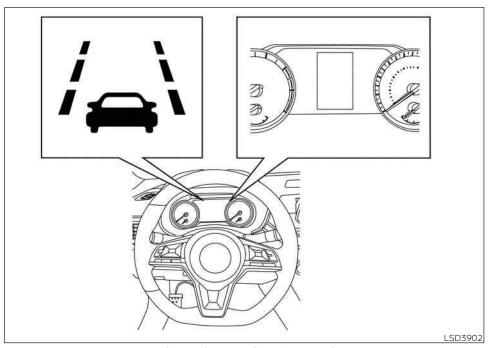
The warning function will stop when the vehicle returns inside of the lane markers.
