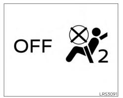
7 If the booster seat is installed in the front passenger seat, place the ignition switch in the ON position. The front passenger air bag status light \*\* \*\* may or may not illuminate, depending on the size of the child and the type of booster seat being used. For additional information, see "Front passenger air bag and status light" (P. 1-55).
