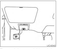
The extended storage switch is used when shipping the vehicle. It is located in the fuse panel to the left of the steering wheel on the instrument panel. If any electrical equipment does not operate, ensure the extended storage switch is pushed fully in place, as shown.
