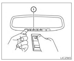
1. Position the end of your hand-held transmitter 1-3 in (2-8 cm) away from the HomeLink® surface, keeping the HomeLink® indicator light (1) in view.
