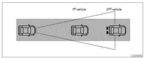
The I-FCW system operates at speeds above approximately 3 mph (5 km/h).
