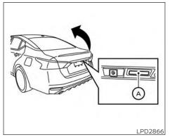
Trunk opener switch (if so equipped)
