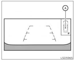
The system indicators (A) will appear when the vehicle moves closer to an object.
