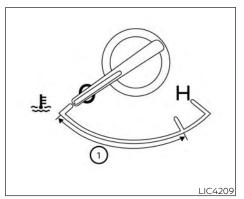
5 inch (13 cm) Type A (if so equipped) **FNGINE COOLANT TEMPERATURE GAUGE**
