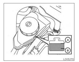
For additional information on brake fluid specification, see "Recommended fluids/ lubricants and capacities" (P. 10-2).
