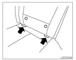
**LATCH** lower anchor location LATCH lower anchor location
