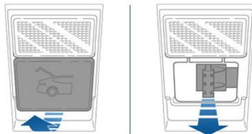
1. Remove the cover by pulling its lower edge very firmly toward you.
