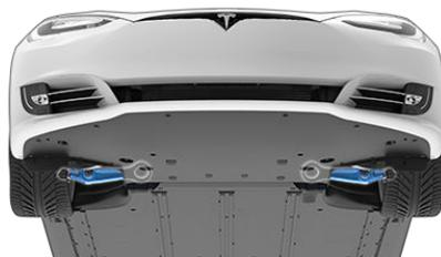
2. To protect the underbody from damage, place a protective barrier (such as a piece of wood) between the tow strap and underbody.
