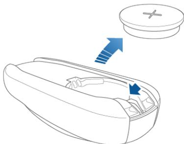
3. Insert the new battery (type CR2354) with the '+' side facing up. The battery fits snugly so you must slide it into position at an angle toward the Positive contact (the contact located near the center of the key), then press down firmly on the other side, ensuring it is held firmly in its intended position.
