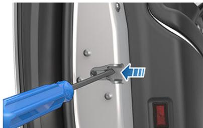
2. Make sure Model X is unlocked, then press the exterior door handle or pull the interior door handle to reset the latch and extend the pop actuator.
