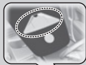
■ Front Wide View Camera Monitors the lane lines
