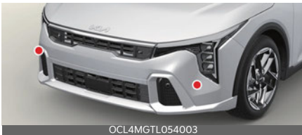
Front corner radar (GT-Line)
