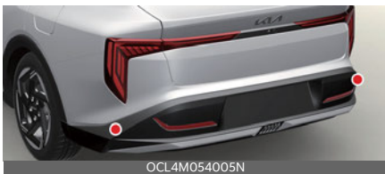
Rear corner radar (GT-Line)
