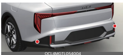
Rear corner radar (GT-Line)
