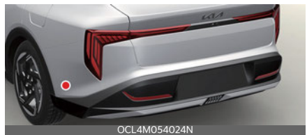
Rear side ultrasonic sensors (GT-Line)
