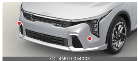
Front corner radar (GT-Line)
