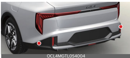
Rear corner radar (GT-Line)
