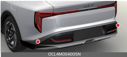
Rear corner radar (GT-Line)
