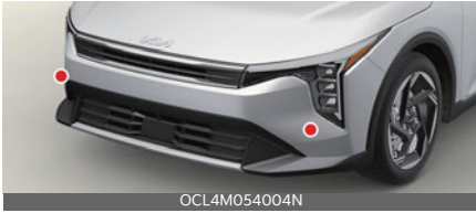
Front corner radar (GT-Line)
