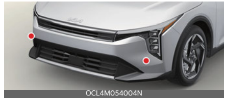
Front corner radar (GT-Line)
