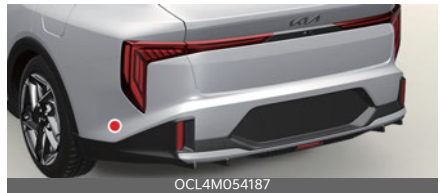
Rear side ultrasonic sensors (GT-Line)
