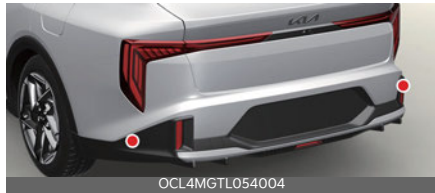
Rear corner radar (GT-Line)
