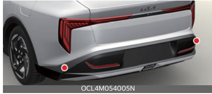
Rear corner radar (GT-Line)
