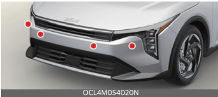
Front ultrasonic sensors (GT-Line)
