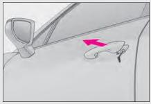
1 Insert the mechanical key while pulling on the driver's door handle.
