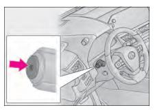
1 Press the Automatic High Beam switch.
