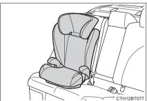
4 Sit the child in the child restraint system. Fit the seat belt to the child restraint system according to the manufacturer's instructions and insert the plate into the buckle. Make sure that the belt is not twisted.
