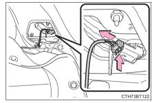
4 Turn the bulb base counter-clockwise.
