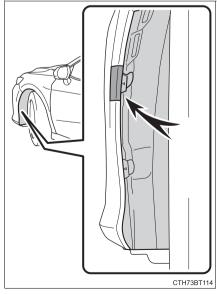
Insert a small flathead screwdriver between the front bumper and fender liner at the position marked with a "∇" and then separate the front bumper from the fender liner
