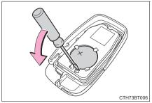
Insert a new battery with the "+" terminal facing up.
