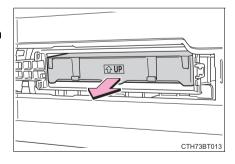
5 Remove the air conditioning filter from the filter case and replace it with a new one.
