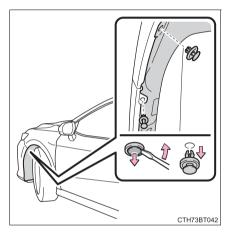
3 To protect the front bumper from being damaged, apply protective tape around the clip as shown in the illustration.
