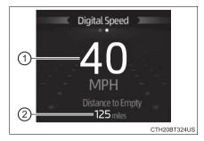
This distance is computed based on your average fuel consumption. As a result, the actual distance that can be driven may differ from that displayed.
