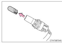
7 Install a new light bulb and then install the bulb base to the light unit by inserting it and turning it clockwise.
