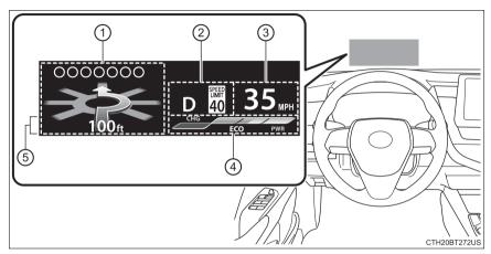
① Driving assist system status/navigation system-linked display area (if equipped) (→P. 138)
