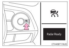
If the cruise control main switch is pressed and held for 1.5 seconds or more, the system turns on in constant speed control mode. (→P. 298)
