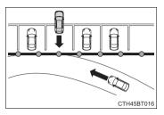
When the distance between your vehicle and metal objects, such as a guardrail, wall, sigh, or parked vehicle, which may reflect electrical waves toward the rear of the vehicle, is short
