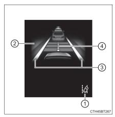
(2) Operation display of steering wheel operation support
