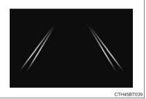
Indicates that the system is recognizing white (yellow) lines or a course\*. When the vehicle departs from its lane, the white line displayed on the side the vehicle departs from flashes yellow.
