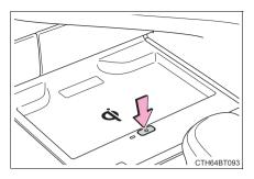
If the power supply switch is pressed 3 times while charging is being performed, the rapid charging function will turn on. To turn the wireless charger off, press the power supply switch when a portable device is not being charged.
