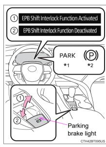
Operate the parking brake switch while depressing the brake pedal.
