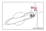
Except for Canada: The trunk is opened using the mechanical key.
