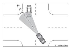
When you turn right/left, pedestrian is detected in the forward direction and estimated to enter your vehicle's (bicyclists path are detected.)
