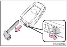
After using the mechanical key, store it in the electronic key. Carry the mechanical key together with the electronic key. If the electronic key battery is depleted or the entry function does not operate properly, you will need the mechanical key. (→P. 527)
