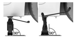
7. Crank the vehicle up, until the vehicle jack is with the entire surface on the ground and the relevant wheel is maximum 1.2 inches/3 cm above ground.
