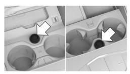
A socket is located between the cup holders in one of the marked positions.
