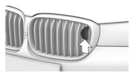
The infrared camera of the Night Vision is located in the radiator grille.
