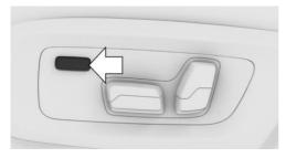
Press the button to reset to standard position.
