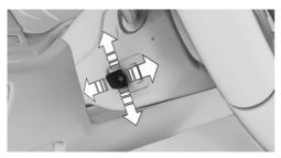
Press the switch to adjust the forward/back position and height of the steering wheel to the seat position.
