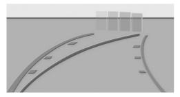
Obstacles behind the vehicle are detected by the PDC Park Distance Control sensors.
