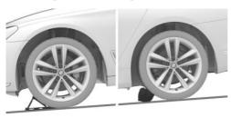
If you need to change a wheel on a slight downhill grade, place chocks and other suitable objects, for instance rocks, under the wheels of both the front and rear axles against the rolling direction.
