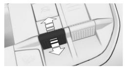
Push the rocker switch forward or pull it back repeatedly until the desired xOffroad driving mode is displayed in the instrument cluster.
