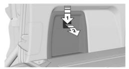
If necessary, remove the cargo cover from the storage under the cargo floor panel.
