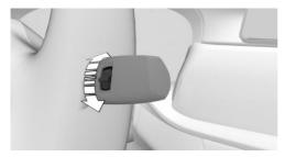
Turn the thumbwheel on the wiper lever.
