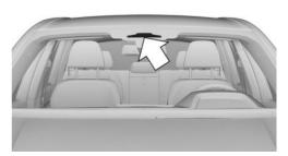
The cameras are located in the area of the interior mirror.
