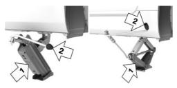
Insert the vehicle jack into the rectangular recess of the jacking point closest to the wheel to be changed.
