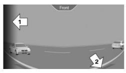
The respective boundary area, arrow 1, in the camera view flashes red, if vehicles are detected by the sensors.
