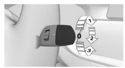
Turn the outer switch upward.
