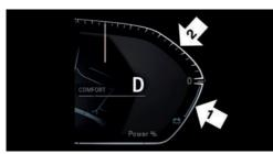
Pointer in the area of arrow 1: display of the energy recovered by coasting or when decelerating, CHARGE.
