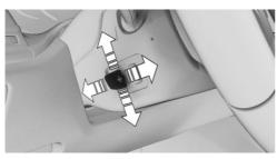
Press the switch to adjust the forward/back position and height of the steering wheel to the seat position.
