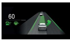
Example: the indicator/warning lights for the Active Cruise Control with Stop & Go function ACC and the Lane Change Assistant indicate a lane change to the next lane. At the same time, the lane change to the next lane is shown with animation in the Assisted Driving View.
