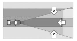
The warning area for the Pedestrian Warning consists of two parts:
