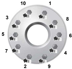
10-wheel nut torque sequence
