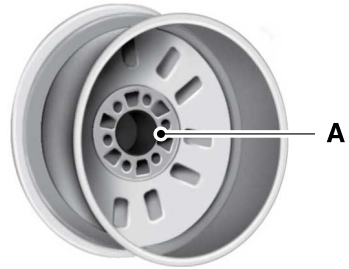
A Hub pilot bore.
