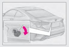
Turn the mechanical key clockwise to open.
