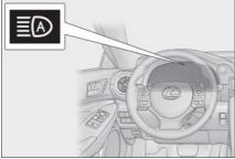
1 Press the Automatic High Beam switch.
