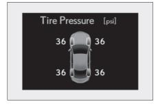
The tire pressure detected by the tire pressure warning system can be displayed on the multi-information display.
