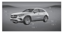
Tire pressure displayed after driving for a few minutes.: current values are not yet known to the system. The pressure/temperature values of each tire are displayed as soon as they are known to the system.
