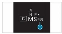
When gearshift recommendation appears on the driver's display, shift to the recommended gear.
