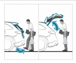
HANDS-FREE ACCESS allows you to open and close the tailgate, or even stop the opening and closing process at any point, by performing a kicking motion under the rear bumper. The transmission must be in position **P** for this function.
