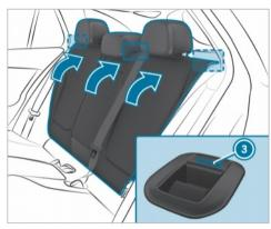
Push seat backrest 2 back to bracket 1 until the backrest engages. If the seat backrest is not engaged and locked in place, red lock verification indicator (3) will be visible.
