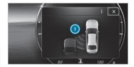
If a course-correcting brake application occurs, the red warning lamp flashes in the outside mirror and a warning tone sounds. In addition, a display
