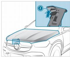
Push handle 2 of the hood catch upwards and lift the hood until it opens automatically.
