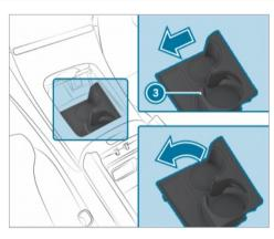
Push the side wall of rear beverage compartment (3) to the left until the cup holder releases and swing the cup holder out upwards.
