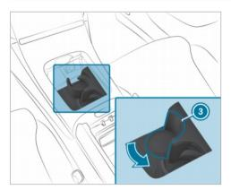
Push the side panel back in the direction of the arrow until it engages in correct position
