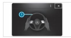
If the system detects that the driver has not steered the vehicle for a considerable period of time or has removed their hands from the steering wheel, an optical warning will be given first. Display 1 will appear on the driver's display. If the driver still does not steer the vehicle, or gives no confirmation to the system, a warning tone will sound in addition to the visual warning message.
