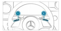
When the automatic transmission is shifted to position D, you can shift it manually with the steering wheel paddle shifters. If permitted, the automatic transmission will shift to a higher or
