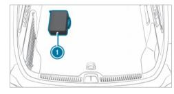
The TIREFIT kit (1) is located on the left-hand side of the cargo compartment in the as-delivered condition.
