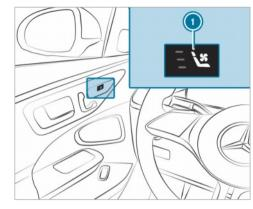
Press button (1) for the respective seat repeatedly until the desired blower setting is reached.
