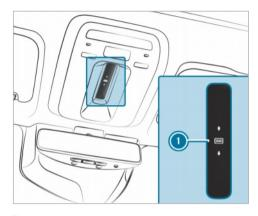
The sliding sunroof and the roller sunblind are operated using control panel ①.
