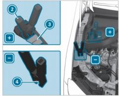
Open cover (3) of positive contact (2) on the jump-start connection point.
