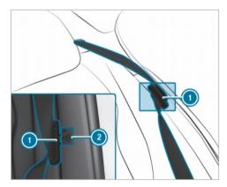
Press the seat belt tongue of seat belt 1 into marked position 2.
