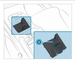
Insert mats (4) in the cup holder beverage compartments can be removed for cleaning.
