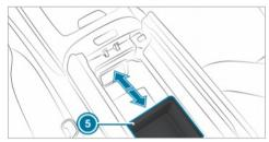
Under armrest ② there is also a sliding storage compartment ⑤, which can be used in the front or rear position. Push the compartment to the desired position until it engages.
