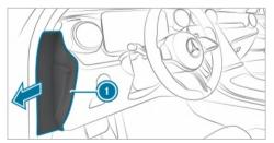
The fuse box is on the driver's side at the side of the cockpit under a cover.
