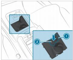
Gently push a beverage container into the bottom 2 of the beverage compartment. The side panel will automatically extend to the left to secure the beverage container.
