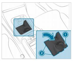
► Insert two lugs ② into the recesses in the trim and swing cup holder ③ into the compartment until it engages.
