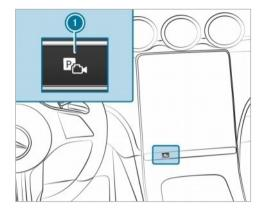
Press button ①. The Camera & Parking view will open on the central display.
