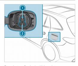
Example: type Combo 1 vehicle socket
