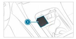
Place the mobile phone in the front storage compartment as centrally as possible with the display facing upwards on mat (1) next to the USB ports.
