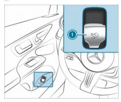
Pull remote operating switch (1) until the tailgate opens.
