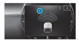
If autonomous braking or situation-dependent brake force boosting has occurred, pop-up 1 will appear on the driver's display and then automatically disappear after a short time.
