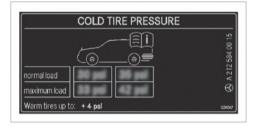
The tire pressure table shows the recommended tire pressure for all tires approved for this vehicle. The recommended tire pressure apply for cold tires under various operating conditions, i.e. loading and/or speed of the vehicle.
