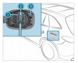
Example:Type Combo 1 vehicle socket
