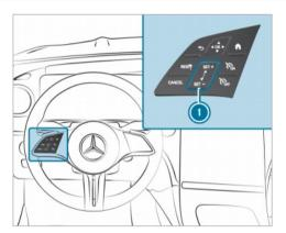
Steering wheel control panel for cruise control
