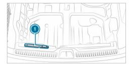
The towing eye (1) is located under the cargo floor in the loading sill.
