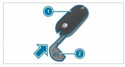
Press emergency key ② into the opening in the key in the direction of the arrow until cover ① opens. When doing so, do not hold cover ① closed.
