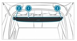
Press in the end cap of cargo compartment cover on the right- or left-hand side.
