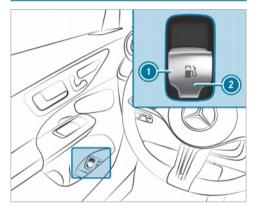
Pull switch (1) once briefly. Indicator lamp (2) will flash and the Please Wait Depressurizing Fuel Tank message will appear on the driver's display.
