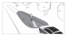
The spotlight function runs in the background and will flash the headlamps in four short bursts at persons detected within the lane markings. You will also be made aware of the position of the person by a projected symbol.
