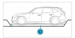
The maximum permissible fording depth ① with roadworthy load is 11.8 in (30 cm).
