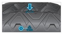
Six marks  $\odot$  show where the bar indicators (arrow) are integrated into the tire tread. They are visible once a tire tread depth of approximately  $V_{16}$  in (1.6 mm) has been reached.
