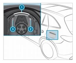
Example: type Combo 1 vehicle socket
