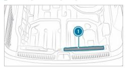
Warning triangle ① is located under the cargo floor in the loading sill when the vehicle is delivered.
