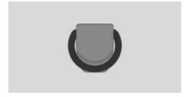
The lashing eyes are located on the loading sill and on the side walls of the cargo area.
