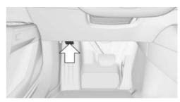
The unlock lever for the hood is located in the driver's footwell.
