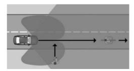
Sensors detect the traffic situation in their detection range when on a straight line.
