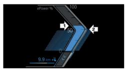
A blue range appears on the power gauge, indicating reduced consumption while driving. Additionally, the bonus range will be displayed. If the blue range turns gray, the fuel consumption has increased.
