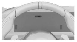
Depending on vehicle equipment, the instrument cluster has one or more infrared light sources. Depending on the light conditions, these light sources can be visible when the vehicle is in standby mode.
