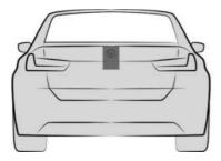
The Rear View Camera is located in the badge on the rear of the vehicle.
