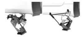
Take your hand away from the jack as soon as the jack is under load and continue turning the jack crank handle or lever with one hand. 5. Make sure that the car jack foot extends vertically and is at a right angle beneath the jacking point.
