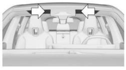
With climate comfort windshield: the marked area is not covered with heat-reflective coating.
