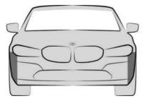
The radar sensors are located on the side of the front bumper.
