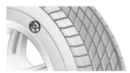
Run-flat tires are indicated by a circular icon containing the letters "RSC" on the tire sidewall.
