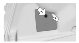
The onboard vehicle tool kit is located in the left storage compartment of the cargo area. Turn the cover lock, arrow 1, and fold out the trim panel, arrow 2.
