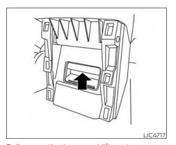
Pull up on the lever and lift up to remove center console.
