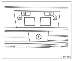
Ensure that the distance sensor (B) is not covered or blocked.
