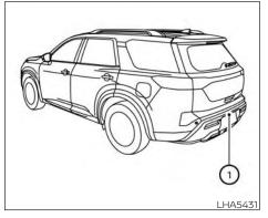
To display the rear view, the Rear View Monitor system uses a camera located in the rear bumper 1.
