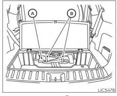
3. Remove the tool kit (A) by releasing the Velcro straps **B**.
