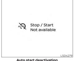
If the engine stops when the Idling Stop System is activated and will not start automatically, the message is shown.
