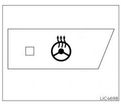
Push the heated steering wheel switch to warm the steering wheel after the ignition switch is placed in the ON position. The indicator light will come on.
