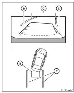
3. Slowly back up the vehicle adjusting the steering wheel so that the predicted course lines (B) enter the parking space
