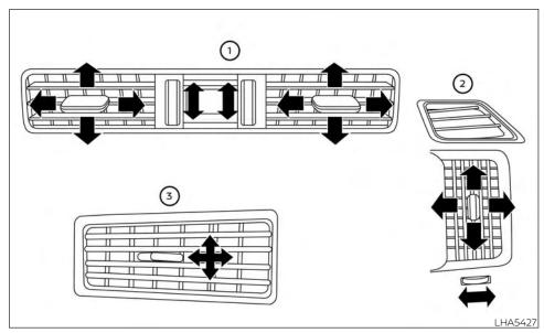
Adjust air flow direction for the center vents ①, driver's and passenger's side vents ②, and rear passenger compartment vents 3 by moving the vent slide and/or vent assemblies.
