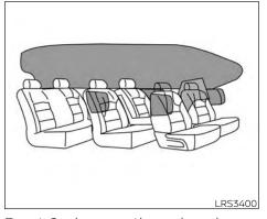
Front, 2nd row outboard, and front central (if so equipped) seat-mounted side-impact supplemental air bag and roof-mounted curtain side-impact and rollover supplemental air bag systems
