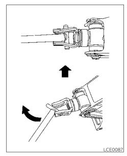
3. Install the assembled jack rod into the jack as shown.
