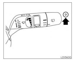
7. Finally, lift the windshield wiper and washer lever to the mist position ① once and release. This action will cause the wipers to resume the set position.
