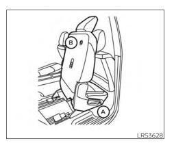
To enter the 3rd row from outside the vehicle, push the seat release button located at the base of the 2nd row seat (A). To exit the 3rd row from inside the vehicle, push the seat release button located on the back of the 2nd row seat (B). Activating this seat release switch will pitch the 2nd row seat forward so you will be able to slide the seat forward and backward
