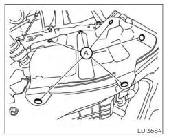
Right engine protector Removal of engine protectors
