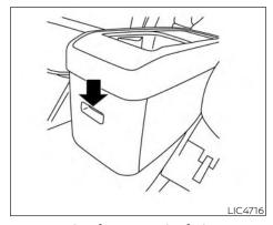
Remove the front panel of the center console.
