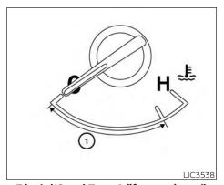
7 inch (18 cm) Type A (if so equipped) **FNGINE COOLANT TEMPERATURE** GAUGE
