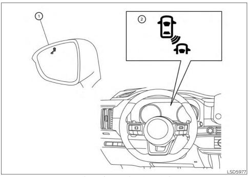
The BSW system operates above approximately 20 mph (32km/h).
