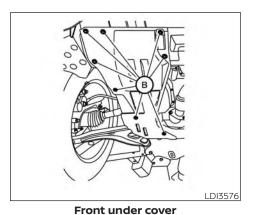
2. Remove pins (B) and front under cover.
