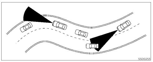
When driving on some roads, such as winding, hilly, curved, narrow roads, or roads which are under construction, the radar sensor may detect vehicles in a different lane, or may temporarily not detect a vehicle traveling ahead. This may cause the I-FCW system to work inappropriately.
