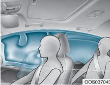
Curtain air bags are located along both sides of the roof rails above the front and rear doors. They are designed to help protect the heads of the front seat occupants and the rear outboard seat occupants in certain side impact collisions.
