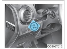
Detach the speed restriction label (1) from the sealant bottle (2), and place it in a highly visible place inside the vehicle such as on the steering wheel to remind the driver not to drive too fast.
