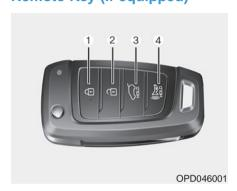
Your HYUNDAI uses a remote key, which you can use to lock or unlock the driver and passenger doors or the rear liftgate.
