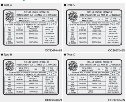
The label located on the driver's door sill gives the original tire size, cold tire pressures recommended for your vehicle, the number of people that can be in your vehicle and vehicle capacity weight.
