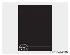
This gauge indicates the current outside air temperature by 1°F (1°C).
