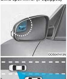
The Blind Spot Mirror (BSM) is a supplemental mirror that minimizes the driver's blind spot zone by expanding the field of view on the
