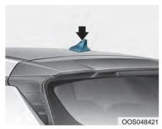
The shark fin antenna receives transmitted data. (for example: AM/FM, SXM, GPS, LTE)
