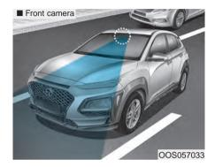
In order for the FCA system to operate properly, always make sure the camera is clean and free of dirt, snow, and debris. Dirt, snow, or foreign substances on the surface may adversely affect the sensing performance of the camera.
