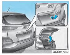
Before attempting to open the liftgate, make sure the vehicle is in PARK (P). To open the liftgate, perform the following:
