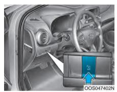
Use the button on the left hand side of the dash panel to activate/deactivate the Head-up display when the ignition is in the ON position or when the engine is running.
