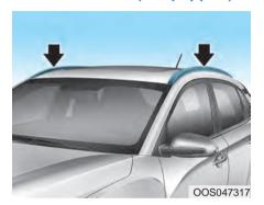
If your vehicle comes equipped with roof side rails, then roof side rails crossbars can be installed on top of your vehicle.
