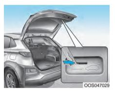
Your vehicle is equipped with an emergency liftgate safety release lever located on the bottom of the liftgate inside the vehicle.
