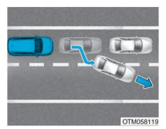
When driving in stop-and-go traffic, and a vehicle in front of you merges out of the lane, the system may not immediately detect the new vehicle that is now in front of you. In this case, you must maintain a safe braking distance, and if necessary, depress the brake pedal to reduce your driving speed in order to maintain a safe distance.
