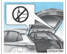
Do not hold on to or try to pull on the liftgate strut. Be aware that the deformation of the liftgate strut may cause vehicle damage and risk of injury.
