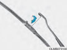
2. Lift up the wiper blade clip (1). Then pull down the blade assembly (2) and remove it.
