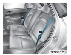
Locate the seatbelt toward the outboard position before folding down the seatback. If not, the seatbelt system may be interfered by the seatback.
