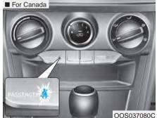
As a reminder to the front passenger, the front passenger's seat belt warning lights will illuminate for approximately 6 seconds each time you place the ignition switch to the ON position regardless of belt fastening.
