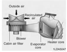
The cabin air filter is installed behind the glove box. It filters the dust or other pollutants that enter the vehicle through the heating and air conditioning system.
