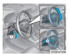
To adjust the steering wheel angle and height:
