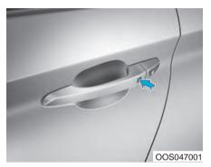
To lock your vehicle using the door handle button or the Smart Key:
