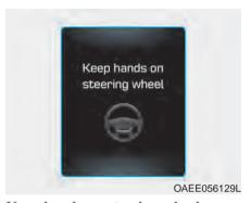
Keep hands on steering wheel If the driver takes their hands off the steering wheel for several seconds while the LKA system is activated, the system will warn the driver.
