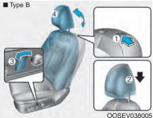
To reinstall the head restraint:
