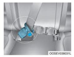
When using the rear center seat belt, the buckle with the "CENTER" mark must be used.
