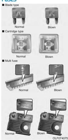
A vehicle's electrical system is protected from electrical overload damage by fuses.
