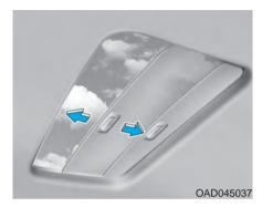
The sunshade can be opened and closed manually. However, the sunshade will open automatically with the sunroof glass when both the sunroof and sunshade are closed and the sunroof control lever is operated.
