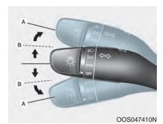
To signal a turn, push down on the lever for a left turn or up for a right turn in position (A).
