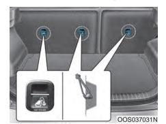
First secure the child restraint with the LATCH lower anchors or the seat belt. If the child restraint manufacturer recommends that the top tether strap be attached, attach and tighten the top tether strap to the top tether strap anchor.
