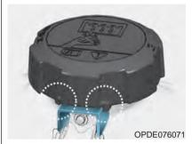
2. Make sure that the tiny protrusions inside the coolant cap is securely interlocked.
