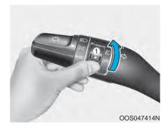
Fog lamps are used to provide improved visibility when visibility is poor due to fog, rain or snow, etc. Use the switch next to the headlamp switch to turn the fog lamps ON and OFF.
