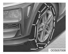
Since the sidewalls of radial tires are thinner than other types of tires, they may be damaged by mounting some types of tire chains on them. Therefore the use of snow tires is preferred over the use of tire chains. If the road and weather conditions require the use of tire chains, be sure to use tire chains that have been properly selected for the size of tire on your HYUNDAI vehicle.
