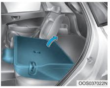
To use the rear seat, lift and unfold the seatback to the upright position. Push the seatback firmly until it clicks into place. Make sure the seatback is locked in place.
