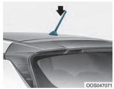
Your vehicle uses a roof antenna to receive AM or/and FM broadcast signals. This antenna pole is removable. To remove the roof antenna pole, turn it counterclockwise.
