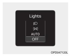
This indicator displays which exterior light is selected using the lighting control.
