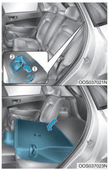
Put out the belt from guide (1) and pull up the seatback folding lever (2), then fold the seat toward the front of the vehicle.
