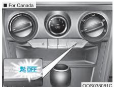
Your vehicle is equipped with an Occupant Classification System (OCS) in the front passenger's seat.
