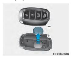
If the Smart Key is not working properly, try replacing the battery with a new one.
