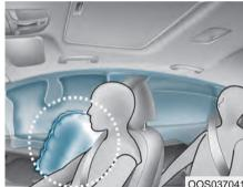
Your vehicle is equipped with a side air bag in each front seat. The purpose of the air bag is to provide the vehicle's driver and the front passenger with additional protection than that offered by the seat belt alone.
