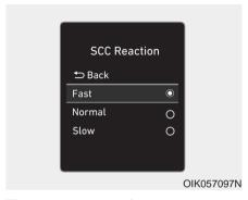
The sensitivity of vehicle speed when following the front vehicle to maintain the set distance can be adjusted. Go to the 'User Settings  $\rightarrow$  Driver Assistance  $\rightarrow$  SCC Reaction  $\rightarrow$  Fast/Normal/Slow' on the LCD display. You may select one of the three stages you prefer.
