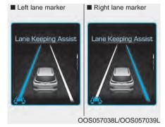
A visual warning appears on the cluster LCD display. Either the left lane line or the right lane line in the cluster LCD display will blink depending on which direction the vehicle is veering.
