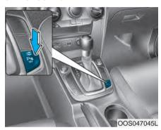
Push the button to turn off the Parking Distance Warning (Reverse) system. The indicator light on the button will turn on.
