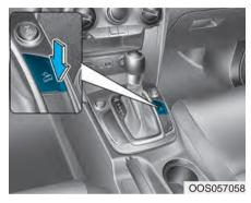
The Downhill Brake Control (DBC) feature assists the driver to descend down a steep hill without having to depress the brake pedal. The system automatically applies the brakes to maintain the vehicle speed below 5 mph (8 km/h) and allows the driver to concentrate on steering the vehicle down hill.
