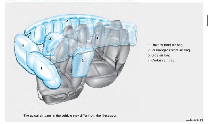
This vehicle is equipped with an Advanced Supplemental Air Bag System for the driver's seat and front passenger's seats.
