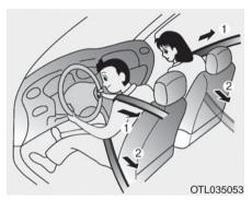
Your vehicle is equipped with driver's and front passenger's Pre-tensioner Seat Belts (Retractor Pretensioner and Emergency Fastening Device System). The purpose of the pre-tensioner is to make sure the seat belts fit tightly against the occupant's body in certain frontal or side collision(s). The Emergency Fastening Device System may be activated in certain crashes where the frontal collision(s) is severe enough, together with the air bags.
