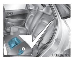
Make sure to insert the belt into the guide (1) and check that the seat belt is not twisted.
