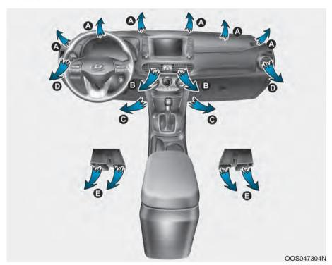
The mode selection knob controls the direction of the air flow through the ventilation system. Air can be directed to the floor, dashboard outlets, or windshield. Five symbols are used to represent Face, Bi-Level, Floor, Floor-Defrost and Defrost air position.
