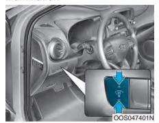
When the vehicle's position lights or headlights are on, press the illumination control button to adjust the brightness of the instrument panel illumination.
