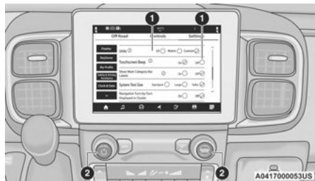
Uconnect 5 NAV With 10.1-inch Display Buttons On The Touchscreen And Buttons On The Faceplate
