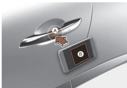
[A] Door handle authentication pad [B] NFC antenna (backside of the smart phone) (The antenna position differs depending on models.)
