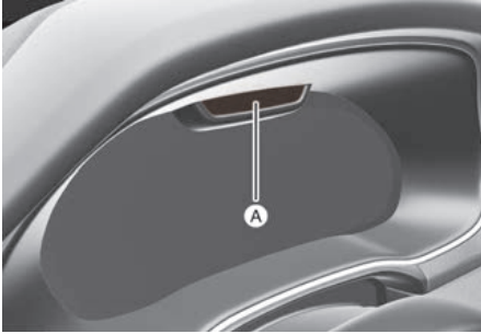
[A] Interior view camera
