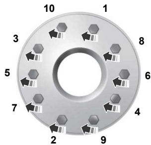
10-lug nut torque sequence.
