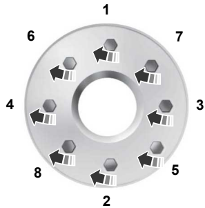
8-lug nut torque sequence.
