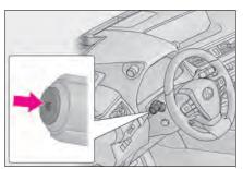
Temporarily switching to the low beams
