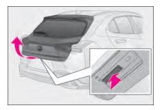
Raise the back door while pressing up the back door opener switch.
