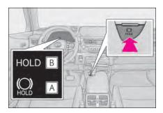
Turns the brake hold system on
