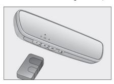
Point the remote control transmitter for the device at the rear view mirror, 1 to 3 in. (25 to 75 mm) from the HomeLink<sup>®</sup> buttons.
