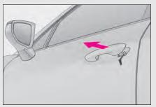
1 Insert the mechanical key while pulling on the driver's door handle.
