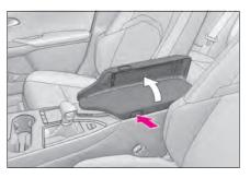
1 Press the button to release the lock and lift the armrest.
