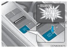
1. With the driver's door and engine hood closed, depress the brake pedal and then press the [AUTO HOLD] switch. The white AUTO HOLD indicator will come on and the system will be in the standby position.
