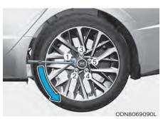
6. Loosen the wheel lug nuts counterclockwise one turn each in the order shown above, but do not remove any lug nuts until the tire has been raised off of the ground.
