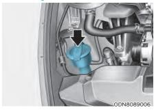
Check the fluid level in the washer fluid reservoir and add fluid if necessary. Plain water may be used if washer fluid is not available. However, use washer solvent with antifreeze characteristics in cold climates to prevent freezing.
