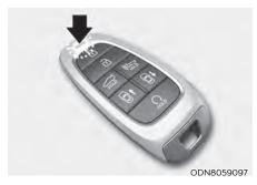
\* When the distance between the smart key and vehicle is over 13 ft. (4 m), the smart key LED may not display normally. You should use it within the operable range.
