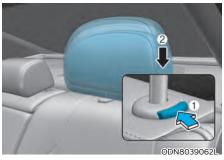
Lower the rear head restraints to the lowest position by pushing and holding the release button and pushing down on the head restraint.
