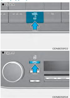
When the ignition switch is in the ON position or when the engine is running, press the heated steering wheel button to warm the steering wheel. The indicator on the button will illuminate.
