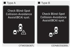
Check Blind-Spot Collision-Avoidance Assist (BCA) system
