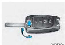
If the remote key does not operate normally, you can lock or unlock the driver's door by using the mechanical key.
