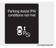
When Remote Smart Parking Assist system is not getting ready for activation, the above message will appear when Remote Smart Parking Assist system button is pressed.
