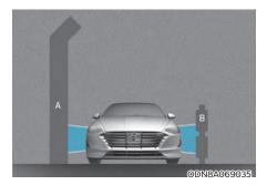
[A]: Noise barrier, [B]: Guardrail
