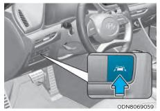
To activate/deactivate LKA system: With the ignition switch in the ON position, press LKA system button located on the instrument panel on the left hand side of the steering wheel.
