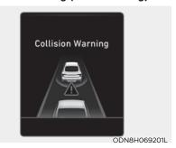
This warning message appears on the LCD display with a warning chime. Additionally, some vehicle system intervention occurs by the engine management system to help decelerate the vehicle.
