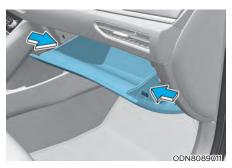
Push in both sides of the glove box as shown. This will ensure that the glove box stopper pins will get released from its holding location allowing the glove box to hang.
