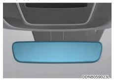
The electric rearview mirror automatically controls the glare from the headlamp of the vehicle behind you in nighttime or low light driving conditions.
