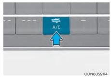
Push the A/C button to turn the system on (indicator light will illuminate) and off.
