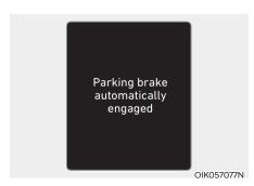
Parking brake automatically engaged If the EPB is applied while Auto Hold is activated, a warning will sound and a message will appear.
