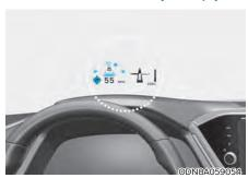
The Head-Up Display is an optional feature that allows the driver to view information projected onto a transparent screen while still keeping your eyes safely on the road ahead while driving.
