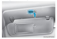
Push the switch to turn the light on or off.
