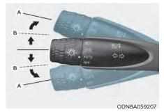
To signal a turn, push down on the lever for a left turn or up for a right turn in position (A).
