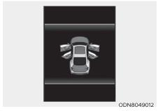
This warning is displayed if any door or the hood or the liftgate is left open. The warning will indicate which door is open in the display.
