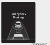
This warning message appears on the LCD display with a warning chime. Additionally, some vehicle system intervention occurs by the engine management system to help decelerate the vehicle.
