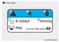
Each symbols and specification on the air conditioning refrigerant label is represented as below:
