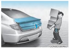
On a vehicle equipped with a smart key, the trunk can be opened using the Smart Trunk with Auto Open system.
