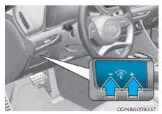
When the vehicle's parking lamps or headlamps are on, press the illumination control button to adjust the brightness of the instrument panel illumination.
