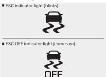
When the ignition switch is placed to the ON position, the ESC indicator light illuminates, then goes off if the ESC system is operating normally.
