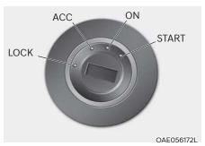
Whenever the front door is opened, the ignition switch will illuminate, provided the ignition switch is not in the ON position. The light will go off immediately when the ignition switch is turned on or go off after about 30 seconds when the door is closed. (if equipped)
