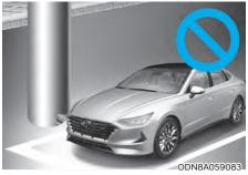
If you want to park your vehicle in the blind spot or near a circular pillar and narrow pillar or a pillar surrounded by objects such as fire extinguisher and the parking distance warning chime sounds three times continuously, the vehicle should not be parked in the area.
