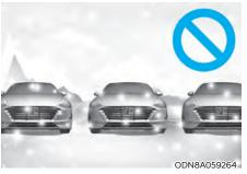
Snow may interfere with sensor operation or Remote Smart Parking Assist system may cancel if the road is slippery while parking.
