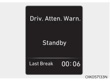
Driver Attention Warning system enters the ready status and displays the 'Standby' screen in the following situations.
