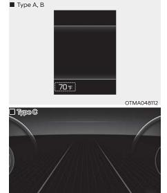
This gauge indicates the current outside air temperature by 1°F (1°C).
