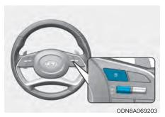
To change the trip mode, toggle the "\,\,\,\" switch on the steering wheel.
