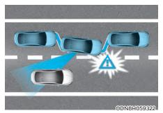
Blind-Spot Collision-Avoidance Assist system detects the front lane through the front view camera installed on the upper front windshield and detects the side/rear areas through rear corner radars.
