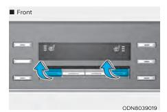
While the engine is running, push either of the switches to warm the driver's seat or front passenger's seat.
