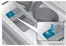
Push the button to turn off Reverse Parking Distance Warning system. The indicator light on the button will turn on.
