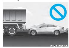
An accident may occur when parking behind a vehicle higher than yours. For example, bus, truck, etc. Do not use the system in that case.
