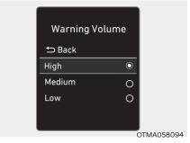
The driver can select the warning volume of Forward Collision Warning in the User Settings in the LCD display or infotainment system display by selecting 'User Settings → Driver Assistance → Warning Volume → High/Medium/Low'.
