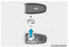
If the Smart Key is not working properly, try replacing the battery with a new one.
