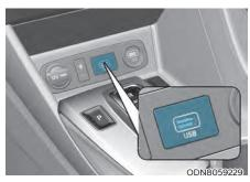
You can use an AUX or USB cable to connect audio devices to the vehicle AUX or USB port.
