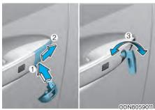
If you lock the driver's door with a mechanical key, all vehicle doors will lock. If you unlock the driver's door with a mechanical key, you can open and close the driver's door only.
