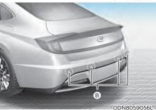
[A]: Front sensor, [B]: Rear sensor
