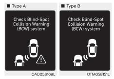
Check Blind-Spot Collision Warning (BCW) system
