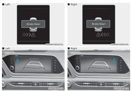
If the risk of collision is detected while RCCW is generated, brake is controlled. The instrument cluster will inform the driver of the brake control. If the rear view monitor system is in activation, a message will also appear on the infotainment system screen.
