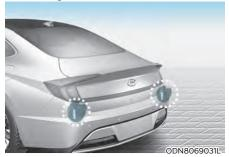
The rear corner radars are sensors located inside the rear bumper to detect the side and rear areas. Always keep the rear bumper clean for proper operation of Safe Exit Assist.
