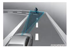
Forward Collision-Avoidance Assist system may recognize a vehicle or pedestrian or cyclist in the next lane or outside the lane when driving on a curved road.
