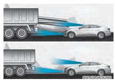
If the vehicle in front of you lif the vehicle in front of you has cargo that extends rearward from the cab, or when the vehicle in front of you has higher ground clearance, additional special attention is required. FCA system may not be able to detect the cargo extending from the vehicle. In these instances, you must maintain a safe braking distance from the rearmost object, and if necessary, depress the brake pedal to reduce your driving speed in order to maintain distance.
