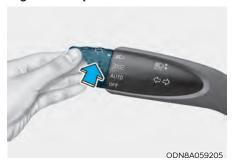
To turn on the high beam headlamp, push the lever away from you. The lever will return to its original position.
