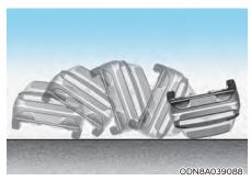
Front air bags may not inflate in rollover accidents because air bag deployment may not provide protection to the occupants.
