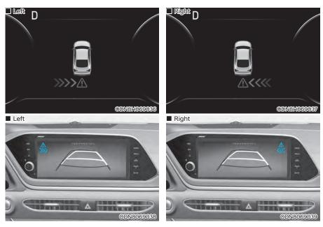
If the vehicle detected by the radar sensors approaches from the rear left/right side of your vehicle, the warning chime will sound, the warning light on the side view mirror will blink and a message will appear on the LCD display or infotainment system display. If the rear view monitor system is in activation, a message will also appear on the infotainment system screen.
