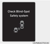
When Safe Exit Assist is not working properly, the 'Check Blind-Spot Safety system' warning message will appear on the cluster, and the system will turn off automatically or the system will be limited. We recommend that the system be inspected by an authorized HYUNDAI dealer.
