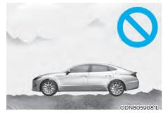
Remote Smart Parking Assist system may cancel when the vehicle slips or the vehicle could not move due to road condition such as pebbles or fragmented stones.
