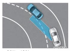
BCW and BCA systems may not operate properly when driving on a curved road. In certain instances, the system may recognize a vehicle in the same lane.
