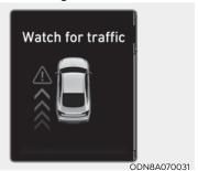
Collision warning when exiting vehicle
