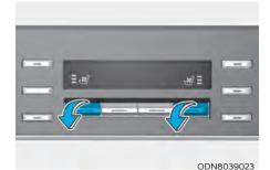
The air ventilation seats are provided to cool the front seats by blowing air through small vent holes on the surface of the seat cushions and seatbacks.
