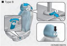
To reinstall the head restraint:
