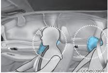
Your vehicle is equipped with a side air bag in each front seat and outboard rear seats. The purpose of the air bag is to provide the vehicle's driver and the front passenger with additional protection than that offered by the seat belt alone.
