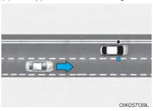
BCW system will alert you when a vehicle is detected approaching in an adjacent lane at a high rate of speed. If the driver activates the turn signal when the system detects an oncoming vehicle, the system sounds an audible alert.
