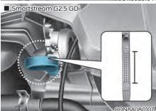
6. Pull the dipstick out again and check the level. The level should be between F and L.
