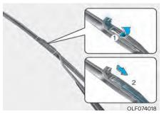
2. Lift the wiper blade clip. Then push down the blade body.
