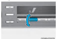
The fan speed can be set to the desired speed by using the fan speed control toggle switch.
