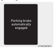
Parking brake automatically engaged When the EPB is applied from Auto Hold, a warning will sound and a message will appear.
