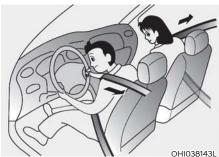
Your vehicle is equipped with driver's and front passenger's Pre-tensioner Seat Belts (Retractor Pre-tensioner). The purpose of the pre-tensioner is to make sure the seat belts fit tightly against the occupant's body in certain frontal or side collision(s).
