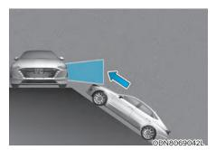
When the vehicle is on/near a slope The system may not operate properly when the vehicle is on/near a slope. In certain instances, the system may not detect the vehicle approaching from the rear left/right and the warning or brake may not operate properly.
