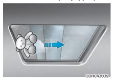
If the sunroof senses any to an obstacle while it is closing automatically, it will reverse direction then stop to allow the object to be cleared.
