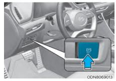
To release the EPB (Electronic Parking Brake):
