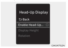
To activate the head up display, select 'Enable Head-Up Display' on the User Settings mode on the instrument cluster LCD display.
