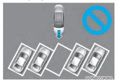
Remote Smart Parking Assist system is not a supplemental for diagonal parking. Even if the vehicle is able to enter the space, do not operate the system.
