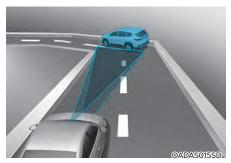
Your vehicle speed can be reduced due to a vehicle in the adiacent lane.
