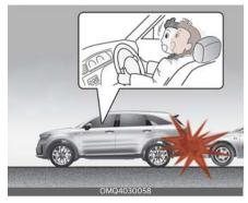
Front airbags may not inflate in side impact collisions, because passengers move in the direction of the collision. Thus, in side impacts, frontal airbag deployment would not provide additional occupant protection.
