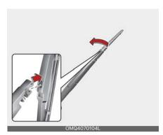
Install the new blade assembly by inserting the center part into the slot in the wiper arm until it clicks into place.
