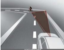
Forward Collision-Avoidance Assist may not detect other vehicles, pedestrians, or cyclists in front of you on curved roads adversely affecting the performance of the sensors. This may result in no warning and braking assist when necessary.
