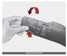
High Beam Assist is a function that automatically adjusts the headlamp range (switches between high beam and low beam) depending on the brightness of detected vehicles and certain road conditions
