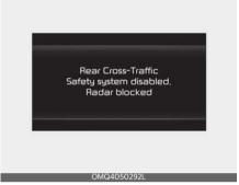
When the rear bumper around the rear corner radar or rear sensor is covered with foreign material, such as snow or rain, or installing a trailer or carrier, it can reduce the detecting performance and temporarily limit or disable Rear Cross-Traffic Collision-Avoidance Assist.
