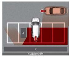
[A]: Structure, [B]: Wall Rear Cross-Traffic Collision-Avoidance Assist may detect vehicles pass-
