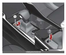
If the shift lever cannot be moved from the P (Park) position into R (Reverse) position with the brake pedal depressed, continue depressing the brake, then do the following:
