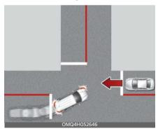
Junction Turning function will help avoid a collision with an oncoming vehicle in an adjacent lane when turning left at a crossroad with the turn signal on by applying emergency braking.
