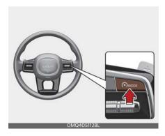
Press the Driving Assist ( MODE) button to turn Cruise Control off. The Cruise ( COLUMN CRUISE) indicator will go off.
