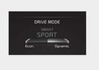
With the standard driving style in the center, the left side of the gauge is 'Econ.' and right side is 'Dynamic' style. When the left side of the driver's style gauge is filled up and after a certain time passes, the SMART ECO mode is activated automatically. When the right side of the gauge is filled up and sporty driving condition is detected, the SMART
