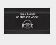
If the driver takes their hands off the steering wheel for several seconds, the 'Keep hands on the steering wheel' warning message will appear on the cluster, and an audible warning will sound in stages.
