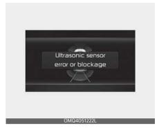
The 'Rear camera error or blockage' or 'Parking sensor error or blockage' warning message will appear on the cluster if the following situations occur:
