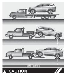
The AWD vehicle should never be towed with the wheels on the ground. This can cause serious damage to the transmission or the AWD system.
