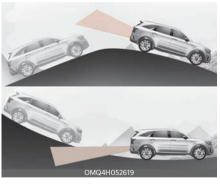
Blind-Spot Safety system may not operate properly when driving on a slope. The function may not detect the vehicle in the next lane or may incorrectly detect the ground or structure.
