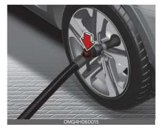
4. Unscrew the valve cap from the valve of the defective tire and screw the filling hose of the sealant bottle onto the tire valve.
