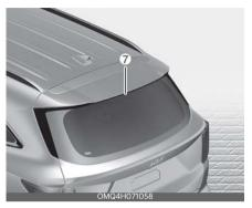
If the high mounted stop lamp (LED) (7) does not operate, have your vehicle checked by an authorized Kia dealer.
