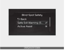
With the ENGINE START/STOP button in the ON position, select 'Driver Assistance → Blind-Spot Safety → Safe Exit Warning from the Settings menu to turn on Safe Exit Warning and deselect to turn off the function.
