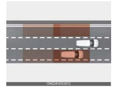
Blind-Spot Collision-Avoidance Assist will help detect and inform the driver that a vehicle is in the blind spot.
