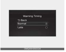
With the ENGINE START/STOP button in the ON position, select 'Driver Assistance → Warning Timing' from the Settings menu to change the initial warning activation time for Rear Cross-Traffic Collision-Avoidance Assist.
