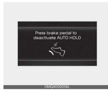
When you press the [AUTO HOLD] switch, if the driver's door and engine hood are not closed, a warning will sound and a message will appear on the LCD display.
