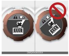
Make sure that the tiny protrusions inside the coolant cap are securely interlocked.
