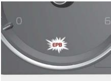
If the EPB malfunction indicator remains on, comes on while driving, or does not come on when the ENGINE START/STOP button is changed to the ON position, this indicates that the EPB may have malfunctioned.
