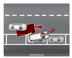
When you are driving forward out of a parking space, if Blind-Spot Collision-Avoidance Assist judges that there is a collision risk with an approaching vehicle in the blind spot, the function will help avoid collision by applying the brake.
