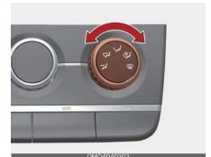
Air can be directed to the floor, dashboard outlets, or windshield. Five symbols are used to represent Face, Bi-Level, Floor, Floor-Defrost and Defrost air position.
