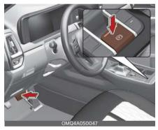
Releasing the parking brake with EPB switch.
