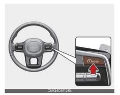
Press the Driving Assist ( MODE) button to turn Manual Speed Limit Assist off. The Speed Limit indicator ( LIMIT) will go off.
