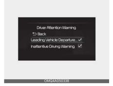
If 'Leading Vehicle Departure Alert' is selected, the function will inform the driver when the front vehicle departs from a stop.
