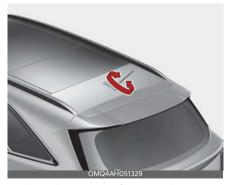
1. Shark fin antenna (Type A, if equipped)
