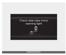
When the side view mirror warning light is not working properly, the 'Check side view mirror warning light' warning message will appear on the cluster. Have the function inspected by an authorized Kia dealer.
