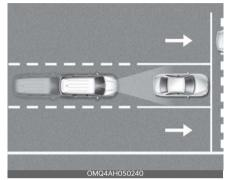
Forward Collision-Avoidance Assist is designed to help detect and monitor the vehicle ahead or help detect a pedestrian in the roadway and warn the driver that a collision is imminent with a warning message and an audible warning, and if necessary, apply emergency braking.
