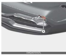
Remove the socket (A) from the assembly by turning the socket counterclockwise until the tabs on the socket align with the slots on the assembly.
