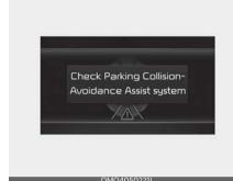
When Reverse Parking Collision- Avoidance Assist or other related systems are not working properly, the 'Check Parking Collision-Avoidance Assist system' warning message will appear on the cluster, and the function will turn off automatically. Have your vehicle inspected by an authorized Kia dealer.
