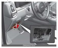
Pull the suspected fuse straight out. Use the removal tool provided in the main fuse box in the engine compartment.
