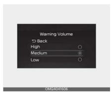
You can adjust the Warning Methods with the ignition switch or ENGINE START/ STOP button in the ON position. With the vehicle on, touch 'Settings → Vehicle → Driver Assistance → Warning Volume' on the infotainment system to change the Warning Methods.
