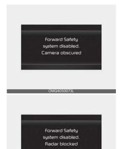
When the front windshield where the front view camera is located, front radar cover, sensor is covered with foreign material, such as snow or rain, it can reduce the detecting performance and temporarily limit or disable Forward Collision-Avoidance Assist.
