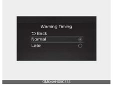
With the ENGINE START/STOP button in the ON position, select 'Driver Assistance → Warning Timing' from the Settings menu to change the initial warning activation time for Forward Collision-Avoidance Assist.
