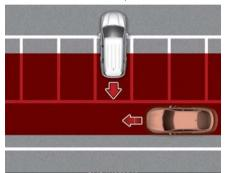
Rear Cross-Traffic Collision-Avoidance Assist may detect vehicles passing by behind you when parking backwards into a parking space. If this occurs, the function may unnecessarily warn the driver and control the brake.
