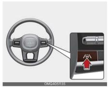
With the ENGINE START/STOP button in the ON position, shortly press the Lane Driving Assist button located on the steering wheel to turn on Lane Following Assist. The white or green ( ) indicator light will appear on the cluster. Press the button again to turn off the function.
