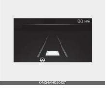
If the vehicle ahead and/or both lane markings are detected and your vehicle speed is above 60 km/h (40 mph) and below 200 km/h (120 mph), the green (a) indicator light will appear on the cluster, and the function will help the vehicle stay in lane by assisting the steering wheel.
