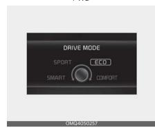
When the Drive Mode is set to ECO mode, the engine and transmission control logic are changed to maximize fuel efficiency.
