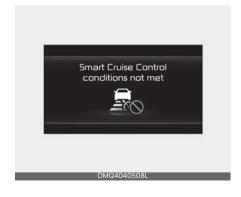
If the Driving Assist ( MODE) button, + switch, - switch or ( ) switch is operated when the function's operating conditions are not satisfied, the 'Smart Cruise Control conditions not met' will appear on the cluster, and an audible warning will sound.
