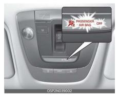
The ODS is designed to detect the presence of a properly-seated front passenger and determine if the passenger's front air bag should be enabled (may inflate) or not. Only the front passenger front air bag is controlled by the ODS. Do not put anything in front of the passenger air bag ( indicator.
