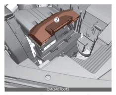
3. Rotate the fixed lever on the filter and loosen the lock.
