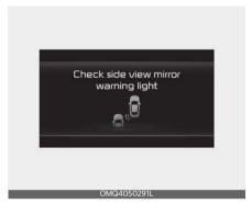
When the side view mirror warning light is not working properly, the `Check side view mirror warning light' warning message will appear on the cluster for several seconds, and the master ( \\_ \text{\Lambda}\)) warning light will appear on the cluster. If the master warning light appears, have the vehicle inspected by an authorized Kia dealer.
