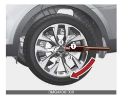
Then position the wrench as shown in the drawing and tighten the wheel nuts. Be sure the socket is seated completely over the nut. Do not stand on the wrench handle or use an extension pipe over the wrench handle. Go around the wheel tightening every other nut until they are all tight. Then double-check each nut for tightness. After changing wheels, have the system checked by a professional workshop. Kia recommends to visit an authorized Kia dealer.
