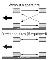
Rotate radial tires that have an asymmetric tread pattern only from front to rear and not from right to left.
