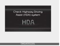
When Highway Driving Assist is not working properly, the 'Check Highway Driving Assist (HDA) system' warning message will appear, and the (\(\bigcarc{\text{1}}{\text{1}}\)) warning light will appear on the cluster. Have the function inspected by an authorized Kia dealer.
