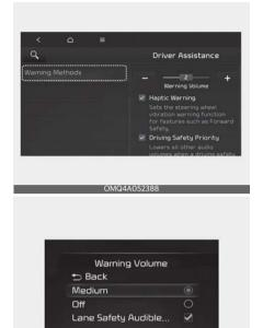
You can adjust the Warning Methods with the ignition switch or ENGINE START/ STOP button in the ON position.
