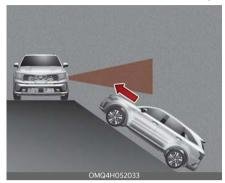
Rear Cross-Traffic Collision-Avoidance Assist may be limited when the vehicle is on a uphill or downhill slope, or near it, and may not detect the vehicle approaching from the left or right. If this occurs, the function may not warn the driver or control the brakes when necessary.
