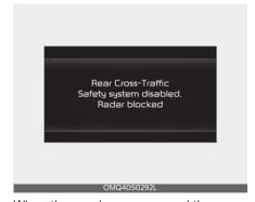
When the rear bumper around the rear corner radar or sensor is covered with foreign matter, such as snow or rain, or
