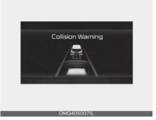
While Smart Cruise Control is operating, when the collision risk with the vehicle ahead is high, the 'Collision Warning' warning message will appear on the cluster, and an audible warning will sound to warn the driver. Always have your eyes on the road while driving, and if necessary, depress the brake pedal to reduce your driving speed in order to maintain a safe distance.
