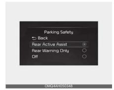
With the ENGINE START/STOP button in the ON position, select or deselect 'Driver Assistance → Parking Safety' from the Settings menu to set whether or not to use each function.
