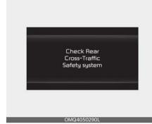
When Rear Cross-Traffic Collision-Avoidance Assist is not working properly, the 'Check Rear Cross-Traffic Safety system' warning message will appear on the cluster, and the function will turn off automatically or the function will be limited. Have the function inspected by an authorized Kia dealer.
