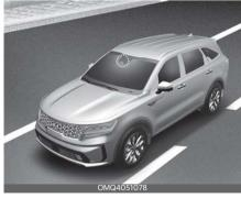
The front view camera is used as a detecting sensor to detect ambient light and brightness while driving. Refer to the picture above for the
