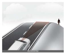
Forward Collision-Avoidance Assist may not detect other vehicles, pedestrians in front of you while driving uphill or downhill adversely affecting the performance of the sensors.
