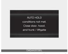
At this moment, press the [AUTO HOLD] button after closing the driver's door and engine hood.
