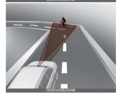
Forward Collision-Avoidance Assist may detect a vehicle, pedestrian, or cyclist in the next lane or outside the lane when driving on a curved road. If this occurs, the function may unnecessarily warn the driver and control the brake. Always check the traffic conditions around the vehicle.
