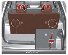
5. To use the rear seat, lift and pull the seatback backward by pulling on the folding lever (for 2nd row) or strap (for 3rd row).
