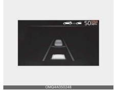
If temporary deceleration is required in the standby state and Navigation-based Smart Cruise Control is operating, the green (AUTO) symbol will appear on the cluster.
