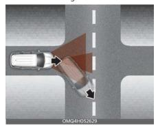
When a vehicle ahead disappears at an intersection, your vehicle may accelerate.
