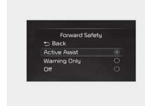
With the ENGINE START/STOP button in the ON position, select or deselect 'Driver Assistance → Forward Safety' from the Settings menu to set whether or not to use each function.
