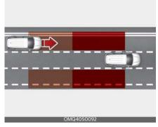
Blind-Spot Collision Assist help detect and informs the driver that a vehicle is approaching at high speed from the blind spot area.
