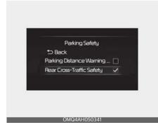
With the ENGINE START/STOP button in the ON position, select 'Driver Assistance → Parking Safety → Rear Cross-Traffic Safety' from the Settings menu to turn on Rear Cross-Traffic Collision-Avoidance Assist and deselect to turn off the function.
