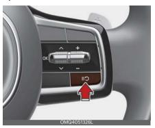
Press the (| ) button to temporarily pause the set speed limit. The set speed limit will turn off but the Speed Limit indicator ( ) IMIT) will stay on.
