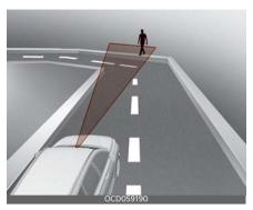
Forward Collision-Avoidance Assist may detect a vehicle, pedestrian in the next lane or outside the lane when driving on a curved road.
