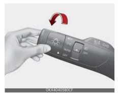
The lights turn on or off depending on the amount of daylight detected from the sensor when the parking brake is not activated or vehicle speed is above 5 km/h (3 mph).
