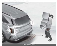
If you are positioned in the detecting area (50 ~100 cm [20 ~ 40 inches] behind the vehicle) carrying a smart key, the hazard warning lights will blink and chime will sound to alert you the smart key has been detected and the liftgate will open.
