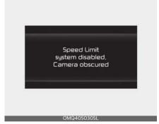
When the front windshield where the front view camera is located is covered with foreign material, such as snow or rain, it can reduce the detecting performance and temporarily limit or disable Intelligent Speed Limit Assist.
