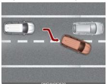
When a vehicle in front of you merges out of the lane, Smart Cruise Control may not immediately detect the new vehicle that is now in front of you.
