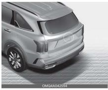
The rear view camera is used as a detecting sensor to detect pedestrians. If the camera lens is covered with foreign
