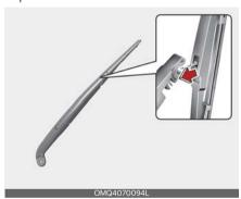
5. Make sure the blade assembly is installed firmly by trying to pull it slightly.
