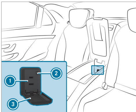
115 V socket in the center console of the rear passenger compartment (Mercedes-Maybach 4-seat vehicles)
