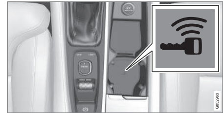
Backup reader's location in the tunnel console.
