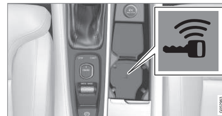
Backup reader's location in the tunnel console.
