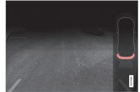
The screen can show coloured sensor fields on the car symbol to the right.
