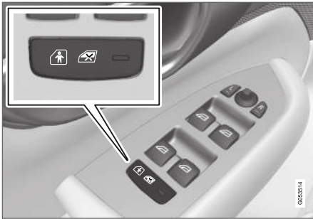
Button for electric activation and deactivation.
