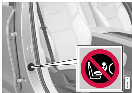
Label on the passenger side's door pillar. The label becomes visible when the passenger door is opened.
