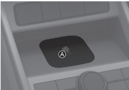
[A] Vehicle authentication pad (Wireless charging pad)
