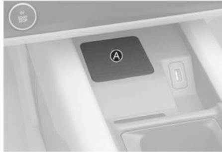
[A] Vehicle authentication pad (Wireless charging pad)
