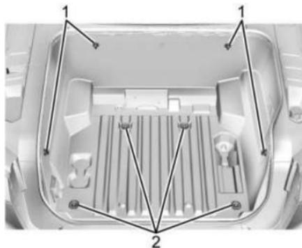
There are four hooks (1) for use with the convenience net, if equipped. The maximum load per hook is 30 kg (66 lbs).
