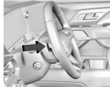
If equipped, Regen on Demand increases deceleration by pressing and holding the steering wheel paddle. Regen on Demand works in D (Drive). The accelerator pedal can be used to manage deceleration while using Regen on Demand. See *One-Pedal Driving* ⇨ 199.
