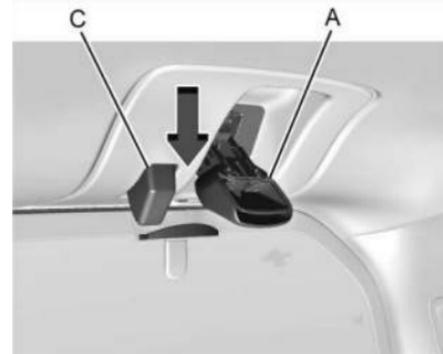
3. Squeeze and pull down the glass latch levers (A), located near the upper corners of the rear glass, to unlatch. Once unlatched, the glass-catch release button (C) will catch the rear glass and prevent it from falling forward.
