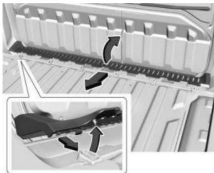
Keep the drain grate clean to avoid blocking the path of water to the gutter system. After hauling dirt, wood chips, pebbles, etc., check the midgate drain to ensure the drain path is clear. The drain grate can be removed and flushed with water if necessary.
