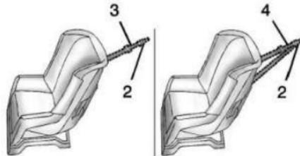
A top tether (3, 4) is used to secure the top of the child restraint to the vehicle. A top tether anchor is built into the vehicle. The top tether attachment hook (2) on the child restraint connects to the top tether anchor in the vehicle in order to reduce the forward movement and rotation of the child restraint during driving or in the event of a crash.
