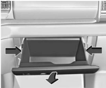
3. Press the sides of the glove box door inward and rotate the door downward to remove.
