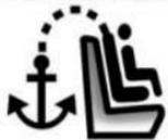
For uplevel models, there are top tether anchor symbols to assist you in locating the top tether anchors.
