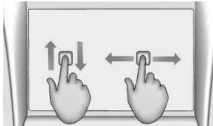
Drag is used to move applications on the infotainment home screen, or to pan the map. To drag the item, it must be held and moved along the display to the new location. This can
