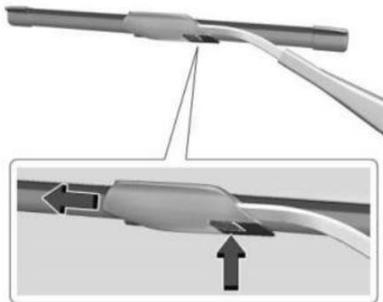
2. Press the button in the middle of the wiper arm connector, and pull the wiper blade away from the arm connector.
