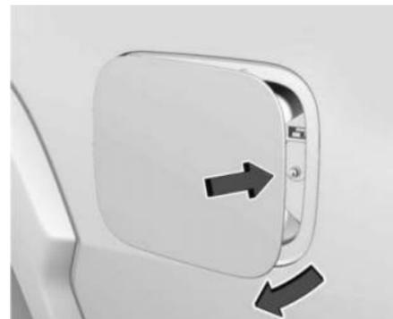
3. Push the rearward edge of the charge port door and release to open the door.
