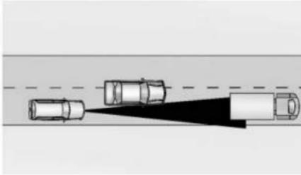
ACC will not detect a vehicle ahead until it is completely in the lane. You may need to manually apply the brakes.
