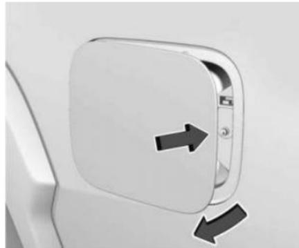
2. The charge port door is on the rear drivers side of the vehicle. Push the rearward edge of the charge port door and release to open.
