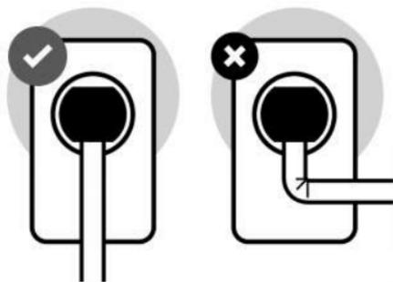
3. Handle electrical cables with care. Do not sharply bend, pull, or crush cables.
