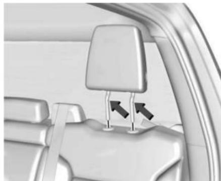
1. Insert the head restraint or headrest posts into the holes in the top of the seatback. The notches on the posts must face the driver side of the vehicle.
