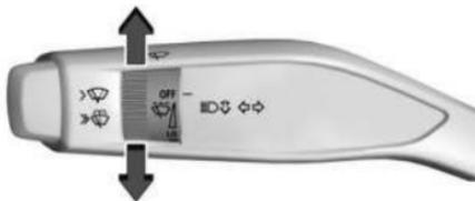
The windshield wiper/washer lever is on the left side of the steering column. With the vehicle on or in accessory mode, move the windshield wiper knob to select the wiper speed.
