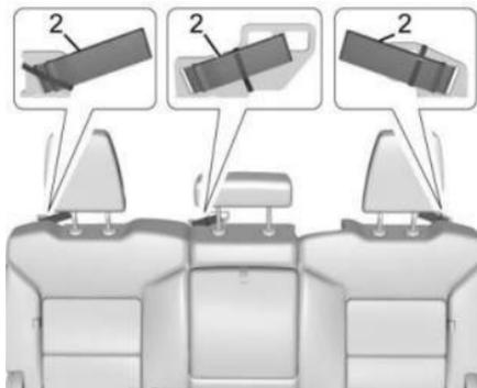
2.1.2 For first time use, remove and discard the rubber band from the top tether loop (2).
