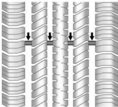
Treadwear indicators are one way to tell when it is time for new tires. Treadwear indicators appear when the tires have only 1.6 mm (1/16 in) or less of tread remaining. See *Tire Inspection* ⇨ 352 and *Tire Rotation* ⇨ 353.
