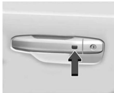
The remote key must be within 1 m (3 ft) of the eTrunk or door being opened or locked. Press the button on the door handle to open. See “Keyless Access Operation” in *Remote Key Operation* ⇨ 9.
