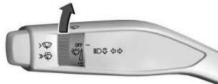
**INT:** Turn the knob to INT for intermittent wipes, then turn the
