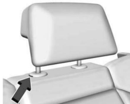
The vehicle's rear seat has adjustable headrest in the center seating position. The headrest can be fully lowered into the seatback to allow for better visibility when the rear seat is unoccupied. When an occupant is in the seat, always pull the headrest up to raise it. Try to move the headrest to make sure that it is locked in place.
