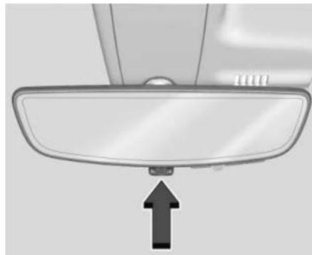
Pull the tab back to turn on the display. Push the tab to turn it off. When off the mirror automatically dims. Adjust the mirror for a clear view of the area behind the vehicle while the display is off.
