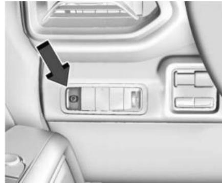
The Electric Parking Brake (EPB) can be applied when the vehicle is on or off. If there is not enough electrical power, the EPB cannot be applied or released. To prevent draining the battery, avoid unnecessary repeated cycles of the EPB.
