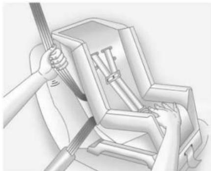
6. To tighten the belt, push down on the child restraint, pull the shoulder portion of the belt to tighten the lap portion of the belt, and feed the shoulder belt back into the retractor.
