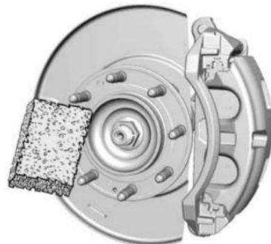
11. Remove any rust or dirt from the wheel bolts, mounting surfaces, and spare wheel.
