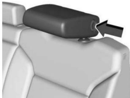
The head restraint can be folded forward to allow for better visibility when the rear seat is unoccupied. To fold the headrest, press the button on the side of the head restraint.
