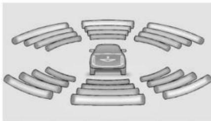
The instrument cluster may have a Park Assist display with bars that show “distance to object” and object location information for the Front and Rear Park Assist system. As the object gets closer, more bars light up and the bars change color from yellow to amber to red.
