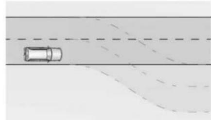
Super Cruise may occasionally provide an alert and/or steering that is considered unnecessary. It could respond to lane markings in different lanes, signs, guardrails, and other stationary objects when entering or exiting a curve. This is normal operation. The vehicle does not need service.
