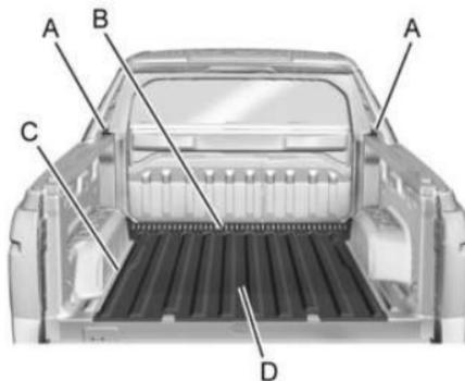
Even when all of these things are working properly and the cover system is on, there may be some instances (heavy rains, automated car washes, etc.) when water can collect in the following areas:
