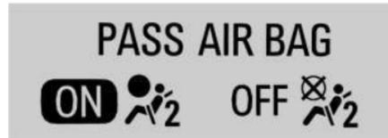
The words ON and OFF will be visible during the system check. When the system check is complete, either the word ON or OFF will be visible. See *Passenger Airbag Status Indicator* ⇨ 114.
