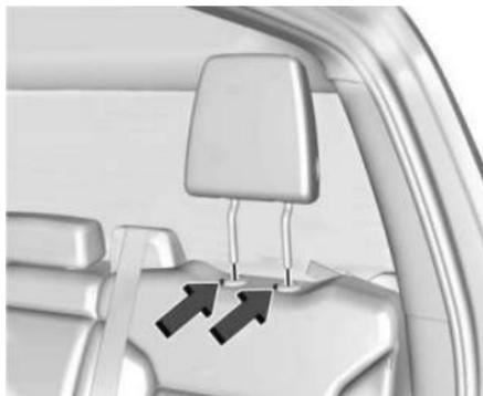
1. Press both buttons on the head restraint or headrest posts at the same time, and pull up on the head restraint or headrest.
