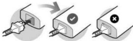
Ensure the connectors are fully inserted into the control box or the charge cord will not work properly.
