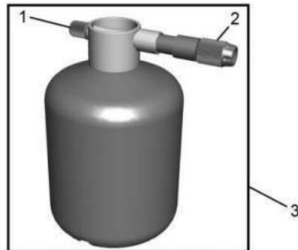
1. Sealant Canister Inlet Valve
