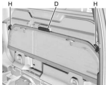
7. Push the glass against the glass stow retainer (D), located on the interior side of the door. Push until the glass handle slides down to lock the glass in place. Close corner secures (H).
