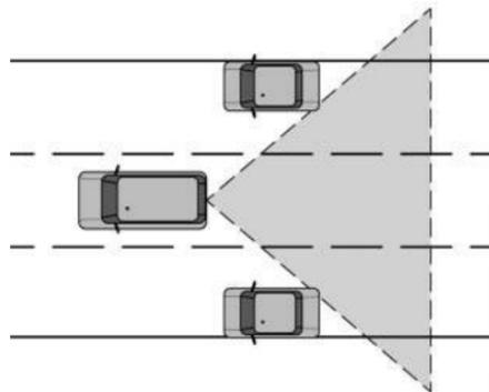
The rear camera mirror provides a wide angle camera view of the area behind the vehicle.
