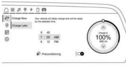
Instead of charging immediately to a desired charge level, you may choose to delay the charge to the vehicle and have it completed by your desired departure time. This may be a more economical choice and a more efficient use of energy when charging at home. To use this mode, touch Charge Later on the Next Charge screen.
