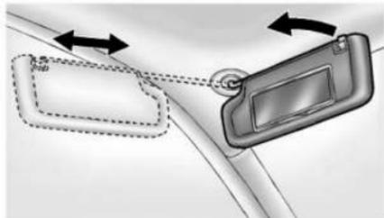
The driver and passenger sun visors can be pulled down to block oncoming glare. If equipped, detach the sun visors from the center mount to pivot to the side window or to extend along the rod.
