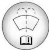
Open the cap with the washer symbol on it. Add washer fluid until the tank is full. See *Underhood Compartment Overview* ⇨ 318 for reservoir location.
