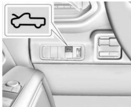
1. To open the hood, press the hood open button on the instrument panel to the left of the steering wheel.
