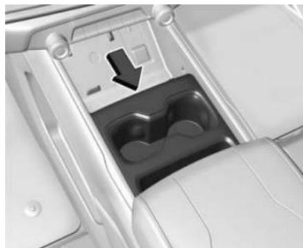
To access additional floor console storage, press the cupholder button and slide the cupholders rearward.
