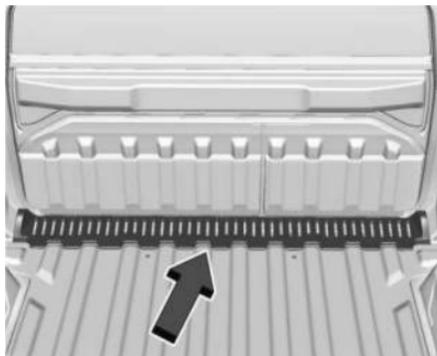
The midgate drain grate is located near the base of the midgate.
