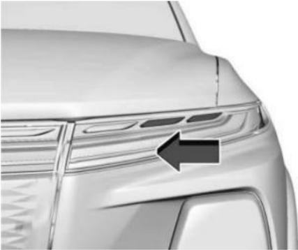
The headlamp CSI bar is located on the headlamps. As charging occurs, the blue light bars on the headlamps fill towards the center of the vehicle.
