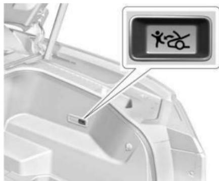
The underhood compartment is equipped with a glow-in-the-dark emergency hood release button. This button will glow following exposure to light. Press the button to open the hood from inside the underhood compartment.
