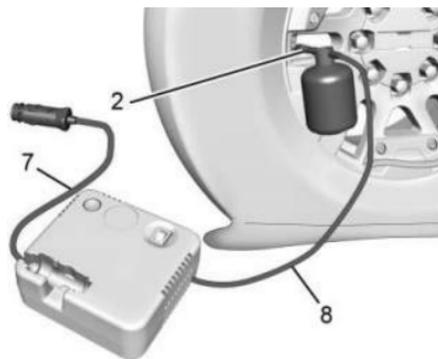
6. Attach the sealant/air hose (2) to the tire valve stem by turning it clockwise until tight.
