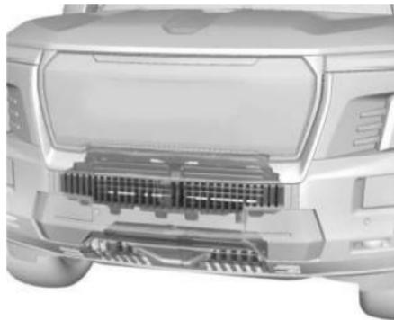
The vehicle may have a shutter system that automatically closes the frontal cooling openings. This system promotes airflow around the vehicle, reducing drag and providing energy savings. Ensure the shutter system is clear of any visible debris, snow, or ice. If the Service Vehicle Soon light activates and remains after clearing the shutter system, see *Service Vehicle Soon Light (Propulsion System Failure)* ⇨ 116.
