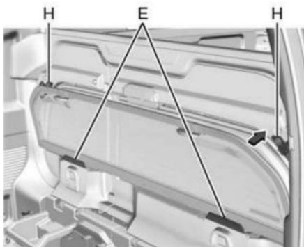
6. Open Corner Secures (H). Load the rear glass into the storage pocket in the midgate, guiding the lower edge of the rear glass behind the two rear glass retaining tabs (E). Hold the rear glass flat against the storage pocket, with grab handles facing you, until the next step.
