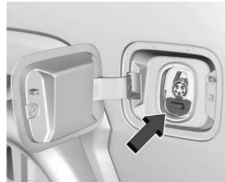
4. Plug in the AC charge cord into the vehicle charge port. Make sure the AC vehicle plug is fully connected to the AC charge port. If it is not properly connected, the vehicle may not be charged.
