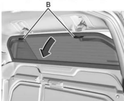
5. With the rear glass tilted toward you, lift it out from the lower window frame channel. Use the grab handles (B) to assist you in removing the rear glass.
