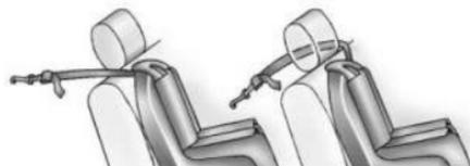
If the position you are using has an adjustable headrest or head restraint, adjust it accordingly to allow proper fitment. If you are using a single tether, route the tether. Make sure the top tether does not interfere with the center seating position shoulder belt/retractor.
