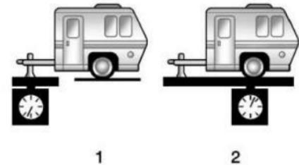
The trailer tongue weight (1) should be 10–15% of the total loaded trailer weight (2). Some specific trailer types, such as boat trailers, fall outside of this range. See the trailer owner's manual for the recommended trailer tongue weight for each trailer. Never exceed the maximum loads for your vehicle, hitch and trailer.
