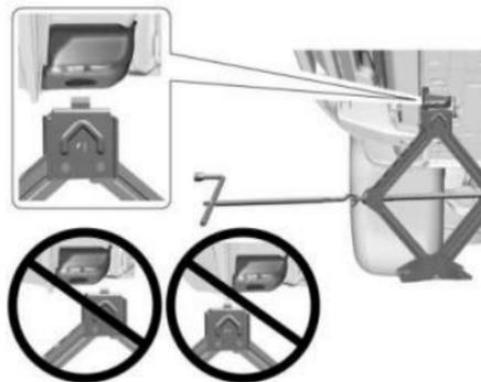
5. Attach the jack handle to the jack by sliding the hook through the end of the jack.
