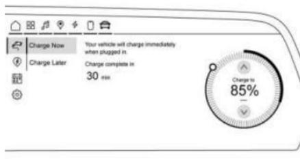
Charge Now is the default charging mode for your vehicle. The vehicle begins charging immediately when it is plugged in and authenticated at the charging location.
