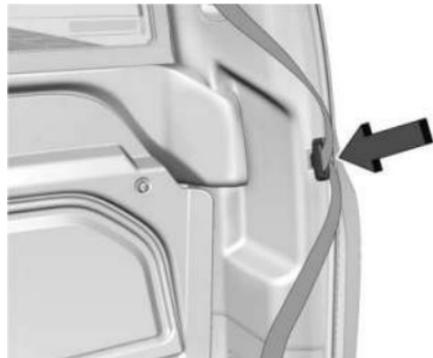
1. Temporarily secure the seatbelt buckle to the opening slot in the door trim to move it out of the path of the midgate.
