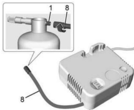
4. Remove the cap from the sealant canister inlet valve (1) by turning it counterclockwise. Attach the air only hose (8) to the sealant canister inlet valve (1) by turning it clockwise until tight.
