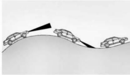
Do not use ACC when driving on steep hills. ACC will not detect a vehicle ahead.
