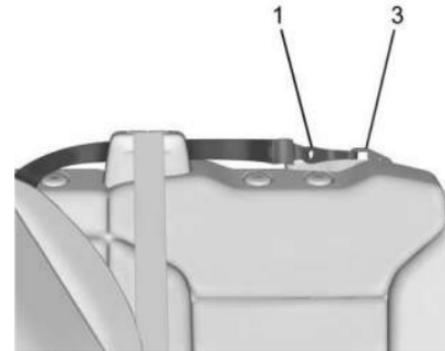
2.3.4 Make sure the child restraint top tether hook is completely closed and secured to the top tether anchor.
