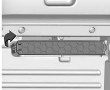
4. Pull lever on left side of the filter door and slide left, then remove the door. Remove the old filter.
