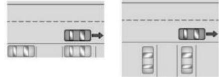
After completely passing an eligible parking spot, a beep sounds and a notification to stop the vehicle is displayed in the driver information center. Generally, APA selects the nearest empty parking spot behind the vehicle, but under some conditions may select a space that is further back. Slow down and bring the vehicle to a complete stop to begin.
