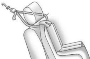
If the position you are using has an adjustable headrest or head restraint, adjust it accordingly to allow proper fitment. If you are using a dual tether, route the tether around the headrest or head restraint posts.
