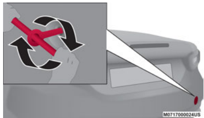
Installing Rear Tow Eye
