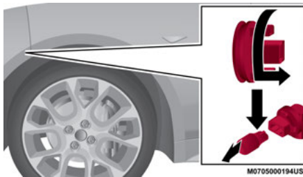
Abarth Direction Indicator Lamp Connector
