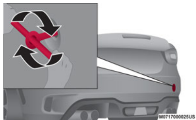
Abarth Installing Rear Tow Eye
