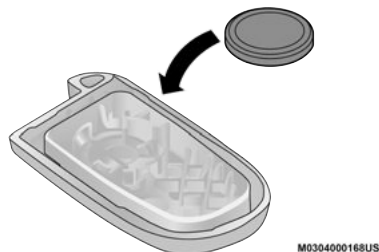
Key Fob Battery Replacement
