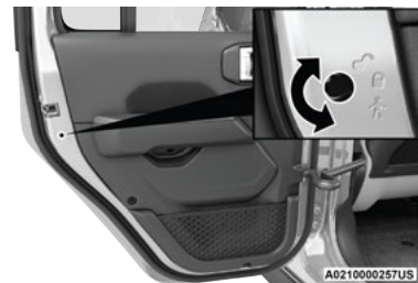
Child-Protection Door Lock Function
