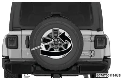
Removing The Spare Tire
