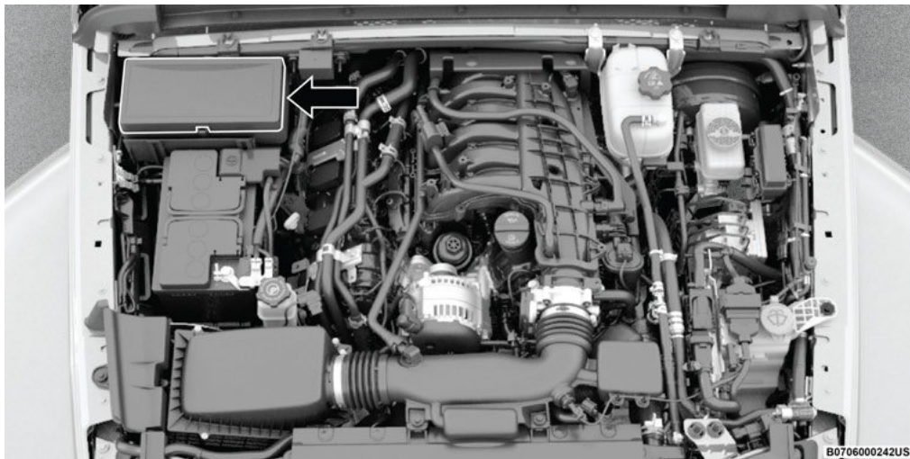
Power Distribution Center Location - Gasoline Engine
