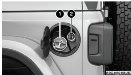
Fuel and Diesel Exhaust Fluid Fill Location
