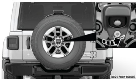
Unlock Rear Camera Cover
