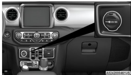
Front Power Outlet
