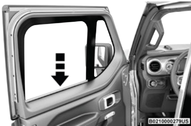
Push Down To Fully Seat Upper Half-Door
