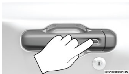
Push The Door Handle Button To Lock
