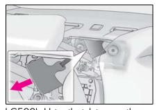
LC500h: Using the tab to open the fuel filler door may not allow for an adequate reduction in fuel tank pressure before refueling. To prevent fuel from spilling out, turn the cap slowly when removing it.
