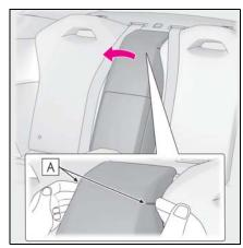
Insert the mechanical key into the cylinder and turn it clockwise to open.
