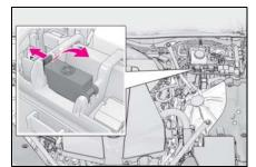
4 Connect a positive jumper cable clamp to A on your vehicle and connect the clamp on the other end of the positive cable to B on the second vehicle.
