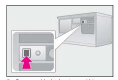
3 Press and hold the desired Home-Link® button (inside the vehicle) for 2 seconds and release it. Repeat this sequence (press/hold/release) up to 3 times to complete programming.
