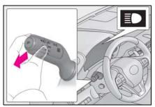
Press the Automatic High Beam switch.
