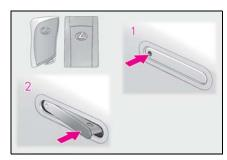
Push the depression on the front edge of the driver's door handle to unlock the door. Push the depression on the front edge of the passenger's door handle to unlock both side doors.\*
