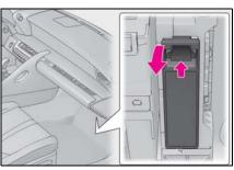
**3** Remove the fuse with the pullout tool.
