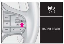
2 Accelerate or decelerate, with accelerator pedal operation, to the desired vehicle speed (at or above approximately 30 mph [50 km/h]) and press the "-SET" switch to set the speed.
