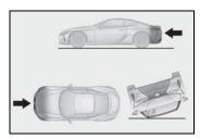
The SRS curtain shield airbags do not generally inflate if the vehicle is involved in a rear collision, if it pitches end over end, or if it is involved in a low-speed side or low-speed frontal collision.
