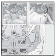
6 Start the hybrid system and turn the air conditioning system on to check that the radiator cooling fan operates and to check for coolant leaks from the radiator or hoses.
