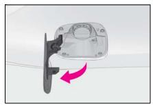
3 Turn the fuel tank cap slowly and remove it, then put it into the holder on the fuel filler door.
