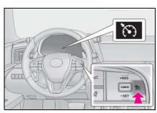
Accelerate or decelerate, with accelerator pedal operation, to the desired vehicle speed (at or above approximately 25 mph [40 km/h]) and press the "-SET" switch to set the speed.
