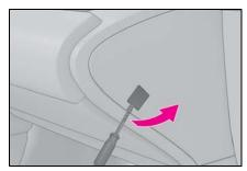
Push the flathead screwdriver into the part shown in the illustration to open the glove box.
