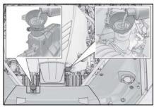
Start the engine and turn the air conditioning system on to check that the radiator cooling fan operates and to check for coolant leaks from the radiator or hoses.
