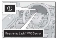
6 Drive the vehicle at 25mph (40 km/h) or more for approximately 10 to 30 minutes.
