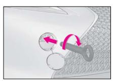
4 Tighten down the towing eyelet securely using the screwdriver or hard metal bar.
