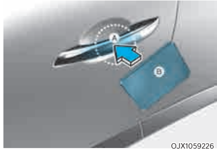
[A] : Door handle authentication pad, [B] : Card key NFC antenna
