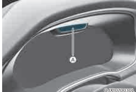
[A] : Interior view camera
