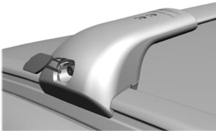
1. Loosen the crossbar bolt by using the supplied tool or similar tool.
