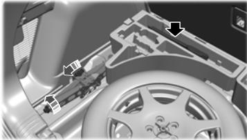
**Note:** On Non Plug-in Hybrid Electric Vehicles, you can find the jack and wrench under the spare tire.
