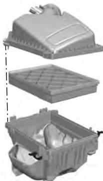
7. Install a new air filter element. Be careful not to crimp the filter element edges between the air filter housing and cover. This could cause filter damage and allow unfiltered air to enter the engine if it is not properly seated.
