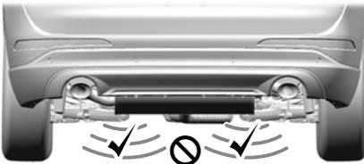
The detection area is on the left-hand side and right-hand side of the hitch, between the exhaust and the hitch.
