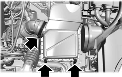
1. Using a screwdriver, loosen the clamp on air filter housing cover.
