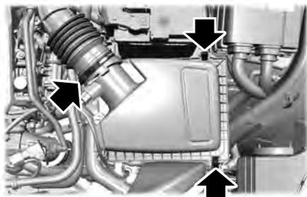
1. Using a screwdriver, loosen the clamp on the air filter housing cover.
