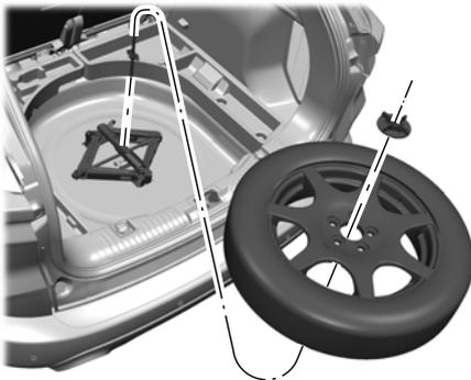
7. Turn the jack hex nut drive screw counterclockwise to detach the lug wrench from the jack. This lowers the jack and releases the mechanical lock.
