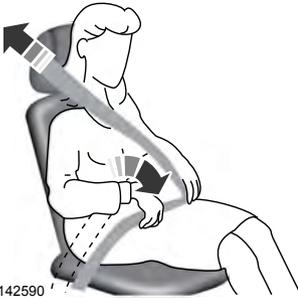
Pregnant women should always wear their seatbelt. Position the lap belt portion of a combination lap and shoulder belt low across the hips below the belly and worn as tight as comfort allows. Position the shoulder belt to cross the middle of the shoulder and the center of the chest.
