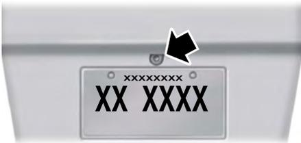
The camera is located on the liftgate.
