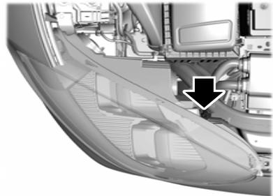
5. Locate the vertical adjuster on each headlamp. Using a Phillips #2 screwdriver, turn the adjuster either clockwise or counterclockwise in order to aim the headlamp. The horizontal edge of the brighter light should touch the horizontal reference line.
