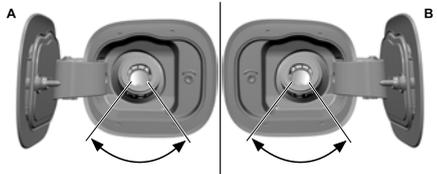
5. Operate the fuel pump nozzle within the area shown.
