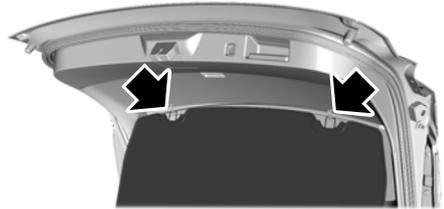
2. Detach the retaining clips on the liftgate trim panel.
