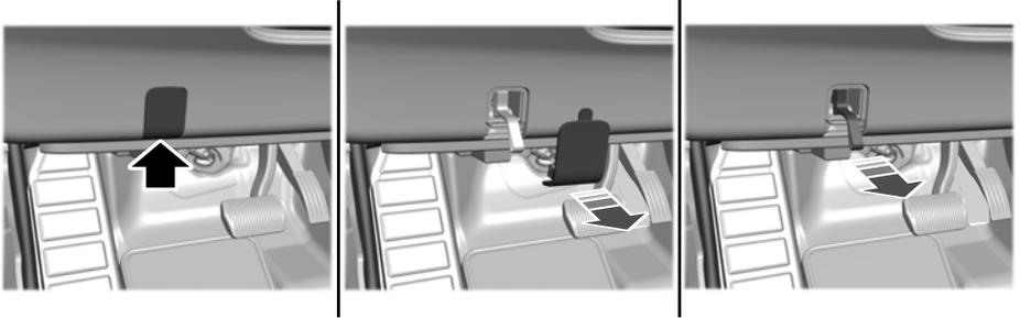
2. Locate the manual park release cable access cover on the lower instrument panel dash to the bottom left hand side of the steering column.
