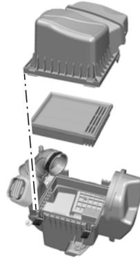
7. Install a new air filter element. Be careful not to crimp the filter element edges between the air filter housing and cover. This could cause filter damage and allow unfiltered air to enter the engine if it is not properly seated.
