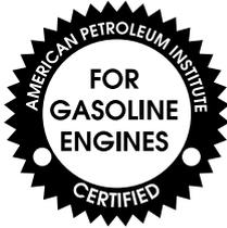
An oil that displays this symbol conforms to current engine, emission system and fuel economy performance standards of ILSAC.
