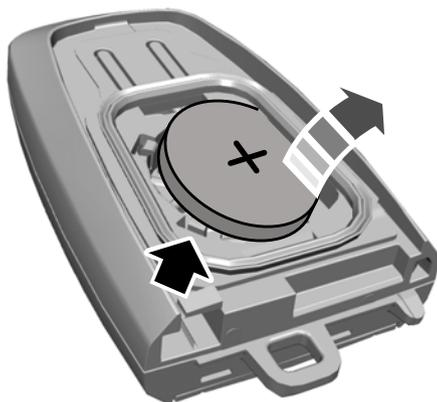
3. Insert a suitable tool, for example a screwdriver, in the position shown and carefully remove the battery.
