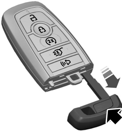
Press the release button and pull the key blade out.
