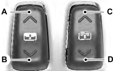
Press and hold the front of the control within two seconds of a bounce-back event to override this function. While bounce-back is active, the closing force increases for each of the next three times that you close the moonroof.
