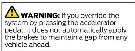
When you press the accelerator pedal, you override the set speed and gap distance.
