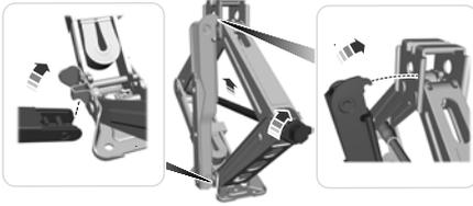
3. Re-position the jack kit assembly into the original vehicle position and secure with the plastic wing nut. Make sure the jack is fastened securely before you drive.
