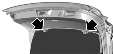
3. Insert the retaining clips into the liftgate trim panel.
