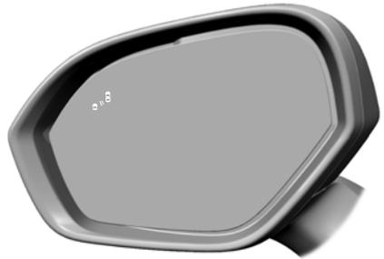
When the system detects a vehicle, an alert indicator illuminates in the exterior mirror on the side the approaching vehicle is coming from. If you turn the direction indicator on for that side of your vehicle, the alert indicator flashes.
