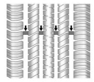
Treadwear indicators are one way to tell when it is time for new tires. Treadwear indicators appear when the tires have only 1.6 mm (1/16 in) or less of tread remaining. See *Tire Inspection* ♀ 296 and *Tire Rotation* ♀ 296.
