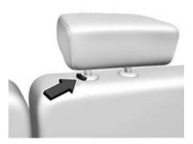
The height of the head restraint can be adjusted. Pull the head restraint up to raise it. Try to move the head restraint to make sure that it is locked in place. To lower the head restraint, press the button, located on the top of the seatback, and push the head restraint down. After releasing the button, ensure the head restraint locks in place and is unable to move up or down.
