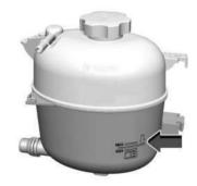
Check to see if coolant is visible in the coolant surge tank. If the coolant inside the coolant surge tank is boiling, do not do anything else until it cools down. If coolant is visible but the coolant level mark is not visible, add a 50/50 mixture of clean, drinkable water and DEX-COOL coolant at the coolant surge tank to the top rib on the middle of the tank, but be sure the cooling system is cool before this is done. See Engine Overheating ♀ 267.
