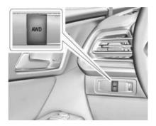
Press the All-Wheel Drive switch to activate the system. The indicator flashes briefly while the system engages and stays lit when the system is active. See *All-Wheel-Drive Light* ▷ 110.
