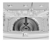
If the vehicle is not equipped with a subwoofer, remove the center wing nut, then remove the spare tire and place it next to the tire being changed.
