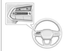
🕥: Press to turn the system on or off. The indicator turns white on the instrument cluster when ACC is turned on.
