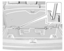
The hold open devices on the cargo bin allow the load floor to remain open without removal.
