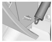
Disconnect the glove box door damper from the glove box door assembly by squeezing the pivot to release the damper ring.
