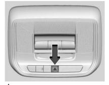
\(\textcal{\textcal{\textcal{\textcal{L}}}}\): Press this button on the overhead console to make the front and rear turn signal lights flash on and off. This warns others that you are having trouble. Press again to turn the flashers off.
