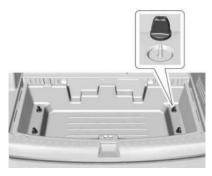
3. Remove the four wing nuts, then remove the cargo management system. See Cargo Management System \$85.
