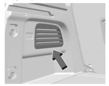
The panel is removed by prying along the top edge of the trim panel. Remove the trim panel to access the fuse block, or see your dealer.
