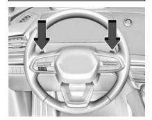
Electronic Range Select, or Manual Mode, allows for the selection of the range of gear positions. Use this mode when driving downhill or towing a trailer to limit the top gear and vehicle speed. The shift position indicator within the Driver Information Center (DIC) will display a number next to the L indicating the highest available gear.
