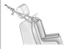
If the position you are using has an adjustable headrest or head restraint, adjust it accordingly to allow proper fitment. If you are using a dual tether, route the tether around the headrest or head restraint posts.
