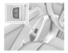
Press on the driver door. The driver door must be unlocked.
