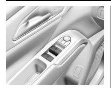
The power windows work when the vehicle is on, in accessory mode, or when Retained Accessory Power is active. See Retained Accessory Power (RAP) ⇒ 185.
