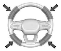
To begin steering manually, hold the steering wheel firmly with both hands using the highlighted regions shown.
