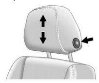
To raise or lower the head restraint, press the button located on the side of the head restraint, and pull up or push the head restraint down, and release the button. After releasing the button, ensure the head restraint locks in place and is unable to move up or down.
