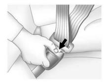
To unlatch the belt, push the pushbutton on the buckle. The belt should return to its stowed position.
