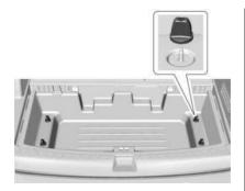
2. Remove the four wing nuts.
