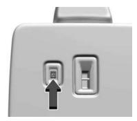
If equipped with power rear seats, the second row seat can also be moved for third row entry/exit by pressing the switch on the second row seat side or on the seatback of the second row seat.
