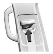
Press and hold the release button while raising or lowering the height adjuster to the desired position.
