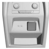
The power outlet is on the rear of the center console
