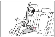
Check that the shoulder belt is correctly positioned over the child's shoulder and that the lap belt is as low as possible.  $(\rightarrow P. 34)$
