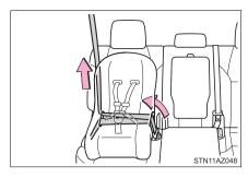
If the child restraint has a top tether strap, the top tether strap should be latched onto the top tether strap anchor. (→P. 70, 73)
