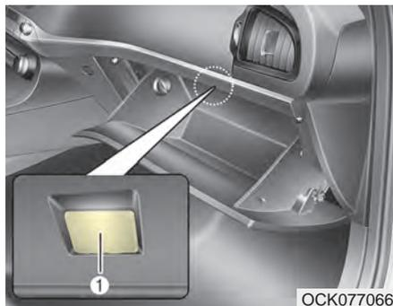
If the glove box lamp (LED) (1) does not operate, have the vehicle checked by an authorized Kia dealer. The LED lamps cannot be replaced as a single component because they are part of an integrated unit. The LED lamps have to be replaced with the unit.
