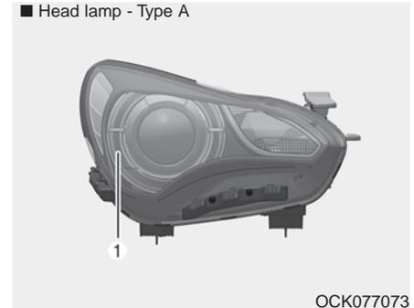
If the position lamp + DRL (LED) (1) does not operate, have the vehicle checked by an authorized Kia dealer.
