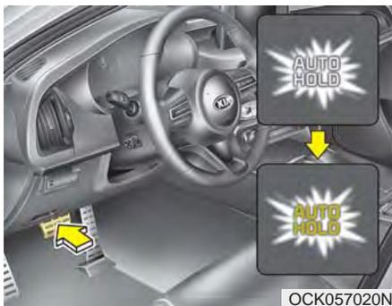
2. When coming to a complete stop by depressing the brake pedal, the AUTO HOLD indicator changes from white to green indicating the AUTO HOLD is engaged. The vehicle will remain at a standstill even if you release the brake pedal.
