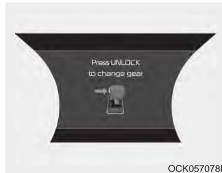
The warning message appears on the LCD display, when the [UNLOCK] button is not pressed while shifting the gear.
