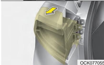
3. Loosen the light assembly retaining screws with a cross-tip screwdriver or spanner.
