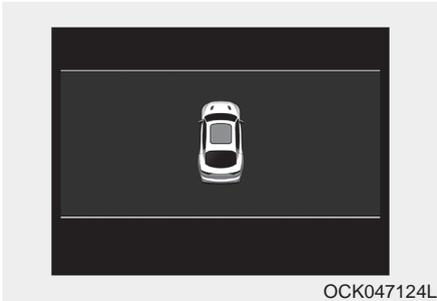
If the driver turns off the engine when the sunroof is not fully closed, the warning chime will sound for a few seconds and the above warning illustration will appear on the LCD display. Close the sunroof securely when leaving your vehicle.
