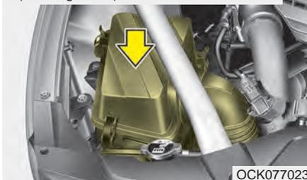
The air filter must be replaced when necessary, and should not be washed.
