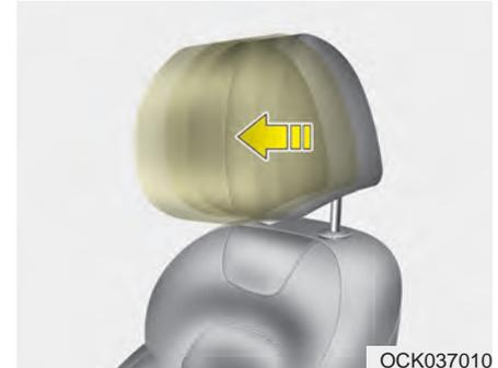
The headrest may be adjusted forward to 4 different positions by pulling the headrest forward to the desired detent.
