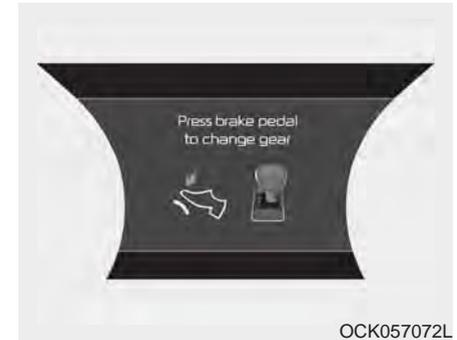
The warning message appears on the LCD display, when the brake pedal is not depressed while shifting the gear.
