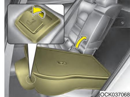
5. To use the rear seat, lift and push the seatback backward. Push the seat back firmly until it clicks into place. Make sure the seatback is locked in place.
