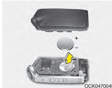
1. Pry open the smart key center cover using screw (-) driver.
