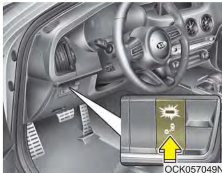
The indicator on the switch will illuminate when the Blind-Spot Collision Warning System (BCW) switch is pressed with the engine start/stop Button ON.
