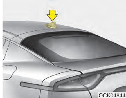
The shark fin antenna will receive both AM and FM signals and the transmit data.
