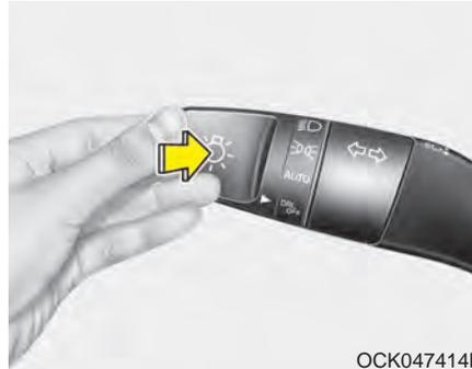
To turn on the high beam headlamp, push the lever away from you. The lever will return to its original position. The high beam indicator will light when the headlight high beams are switched on.
