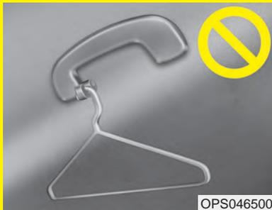
**Do not hang other objects such as hangers or hard objects except clothes. Also, do not put heavy, sharp or breakable objects in the pockets of the clothing. In an accident or when the curtain air bag is inflated, it may cause vehicle damage or personal injury.**
