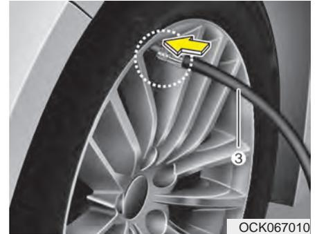
6. Unscrew the valve cap from the valve of the defective wheel and screw filling hose (3) of the sealant bottle onto the valve.
