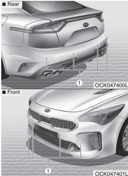
The parking distance warning-forward assists the driver during movement of the vehicle by chiming if any object is sensed within the distance of 39 in. (100 cm) in front and 47 in. (120 cm) behind the vehicle.
