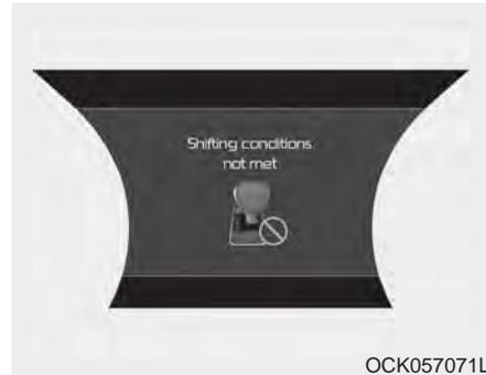
The warning message appears on the LCD display, when engine RPM is too high, or when driving speed is too fast to shift the gear.
