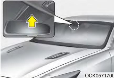
The Lane Keeping Assist (LKA) system is designed to detect the lane markers on the road with a front view camera at the front windshield, and assists the driver's steering to help keep the vehicle in the lanes.
