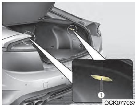
If the luggage room lamp (LED) (1) does not operate, have the vehicle checked by an authorized Kia dealer. The LED lamps cannot be replaced as a single component because they are part of an integrated unit. The LED lamps have to be replaced with the unit.
