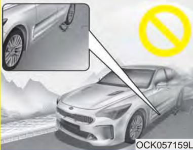
**Never start or run the engine while an AWD vehicle is raised on a jack. The vehicle can slip or roll off of a jack causing serious injury or death to you or those nearby.**
