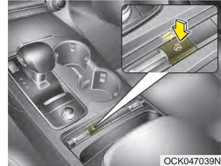
With the Engine Start/Stop Button in the ON position, pressing the heated steering wheel button warms the steering wheel. The indicator on the button will illuminate.
