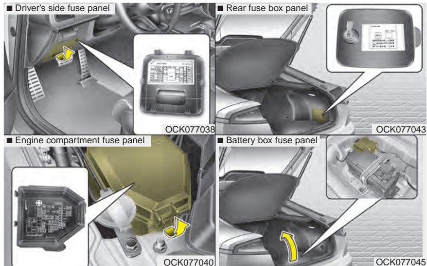
Inside the fuse/relay panel covers, you can find the fuse/relay label describing fuse/relay name and capacity.
