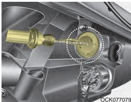
3. Remove the bulb-socket from the headlamp assembly by turning the bulb-socket counterclockwise until the tabs on the bulb-socket align with the slots on the headlamp assembly.
