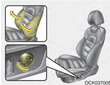
1. Turn the adjustment switch clockwise, the right/left seatback bolsters will be adjusted inward. Turn the switch counterclockwise, the seatback bolster will be adjusted outward.
