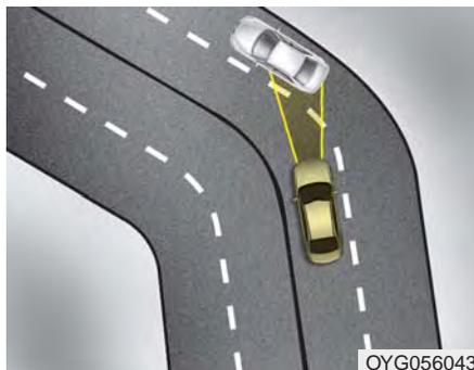
The FCA system may recognize a vehicle in an adjacent lane when driving on a curved road. In this case, the system may apply the brake. Always pay attention to road and driving conditions while driving. If necessary, depress the brake pedal to reduce your driving speed in order to maintain a safe distance. Also, when necessary, you may depress the accelerator pedal to prevent the system from unnecessarily decelerating your vehicle. Always check the traffic conditions around the vehicle.
