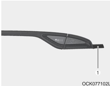
If the rear side marker (LED) (1) does not operate, have the vehicle checked by an authorized Kia dealer. The LED lamps cannot be replaced as a single component because they are part of an integrated unit. The LED lamps have to be replaced with the unit.
