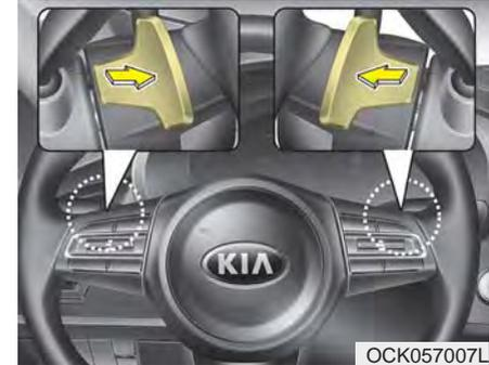
The paddle shifter is available when the shift lever is in the D position or the manual mode.
