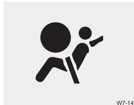
The purpose of air bag warning light in your instrument panel is to alert you of a potential problem with your air bag system, which could include your side and/or curtain air bags used for rollover protection.
