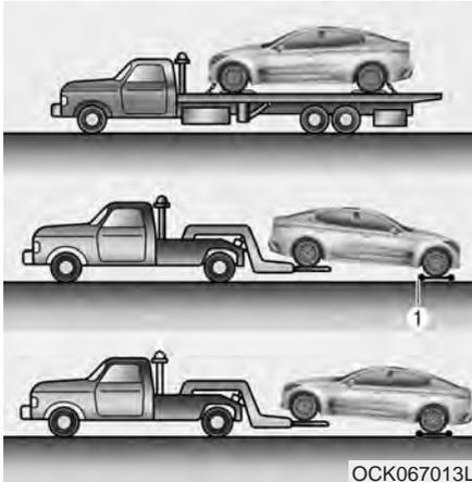
If emergency towing is necessary, we recommend having it done by an authorized Kia dealer or a commercial tow-truck service. Proper lifting and towing procedures are necessary to prevent damage to the vehicle. The use of wheel dollies(1) or flatbed is recommended.
