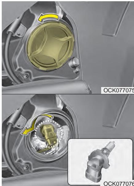
2. Remove the headlamp bulb cover by turning it counterclockwise.
