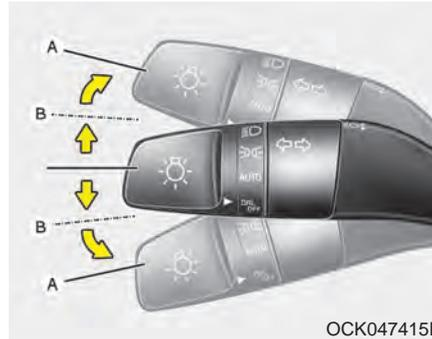
The ignition switch must be on for the turn signals to function. To turn on the turn signals, move the lever up or down (A). The green arrow indicators on the instrument panel indicate which turn signal is operating.
