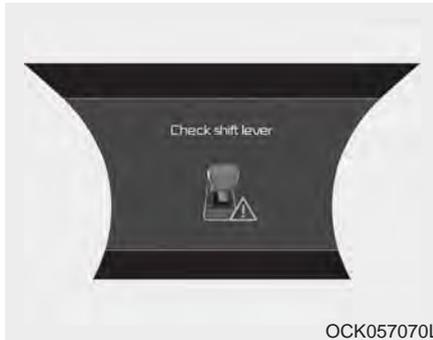
The warning message appears on the LCD display, when there is a malfunction with one of the key transmission components.
