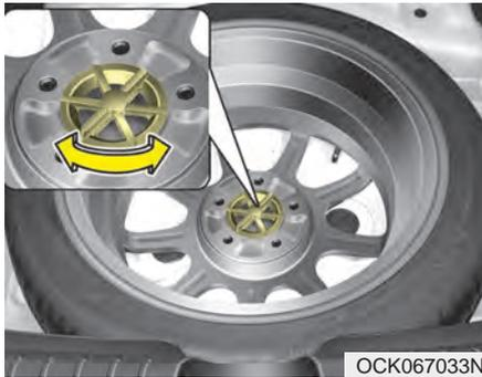
Turn the tire hold-down wing bolt counterclockwise.
