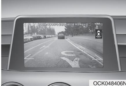
The rear view monitor will activate with the ignition switch ON, engine ON and the shift lever in the R (Reverse) position.
