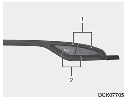
If the stop and tail lamp (LED) (1, 2) does not operate, have the vehicle checked by an authorized Kia dealer. The LED lamps cannot be replaced as a single component because they are part of an integrated unit. The LED lamps have to be replaced with the unit.
