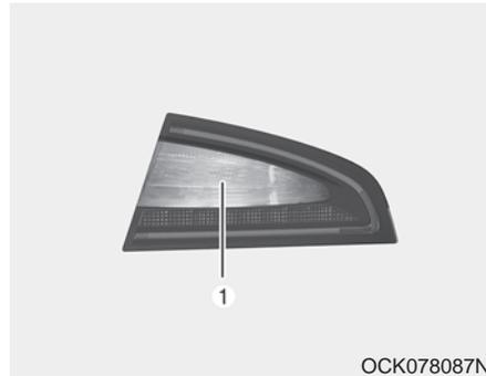
If the rear turn signal lamp (LED) (1), does not operate, have the vehicle checked by an authorized Kia dealer. The LED lamps cannot be replaced as a single component because they are part of an integrated unit. The LED lamps have to be replaced with the unit.
