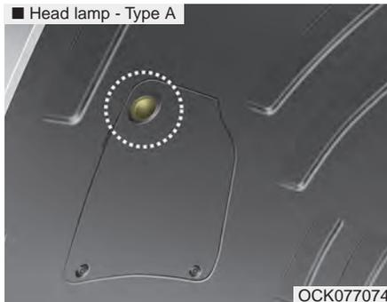
1. Remove the service cover clip on the wheel housing.
