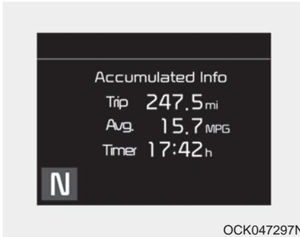
Displays accumulated information starting from mileage/fuel efficiency/time default point.
