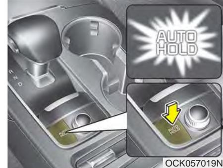
1. Depress the brake pedal, start the engine and then press the Auto Hold button. The white AUTO HOLD indicator will come on indicating the system is in standby.
