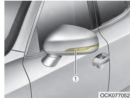
If the side repeater lamp (LED) (1) does not operate, have the vehicle checked by an authorized Kia dealer. The LED lamps cannot be replaced as a single component because they are part of an integrated unit. The LED lamps have to be replaced with the unit.
