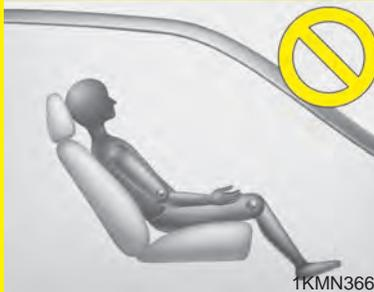
The driver must advise the passengers to keep the seatback in an upright position whenever the vehicle is in motion. If a seat is reclined during an accident, the restraint system's ability to restrain will be greatly reduced.
