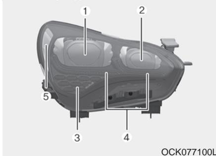
If the Low/High beam lamp (1, 2), Front turn signal lamp (3), Day time running lamp/Position lamp (4), and/or Side marker (5) do not operate, have the vehicle checked by an authorized Kia dealer.
