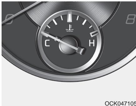
This gauge indicates the temperature of the engine coolant when the Engine Start/Stop button is ON.
