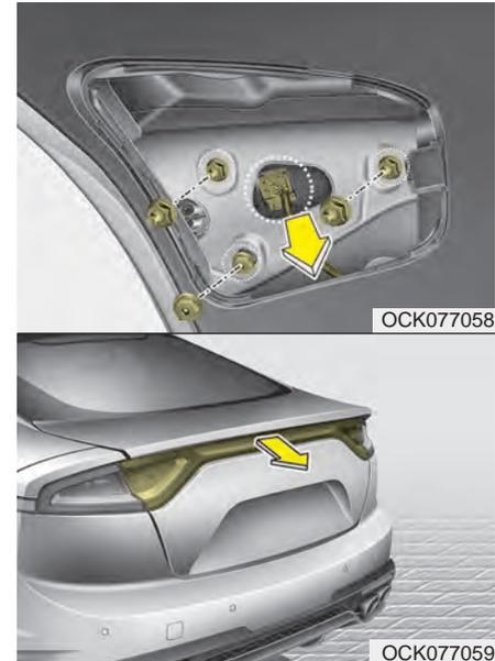
3. Remove the nuts from rear combination lamp of both side (drive side and passenger side).
