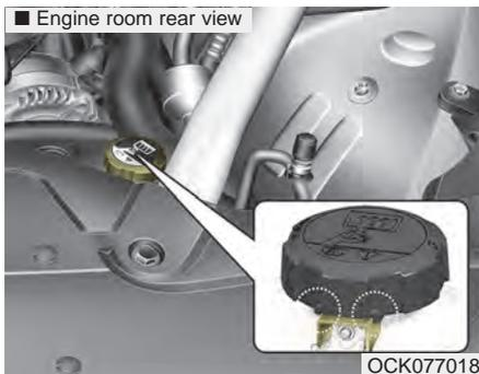
2. Make sure that the tiny protrusions inside the coolant cap are securely interlocked.
