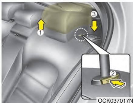
**Adjusting the height up and down (if equipped)**
