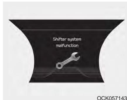
The warning message appears on the LCD display, when the transmission or the shift lever does not properly operate in the P (Park) position. In this case, have the vehicle inspected by an authorized Kia dealer immediately.
