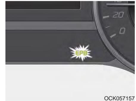
This warning light illuminates if the engine start/stop button is changed to the ON position and goes off in approximately 3 seconds if the system is operating normally.
