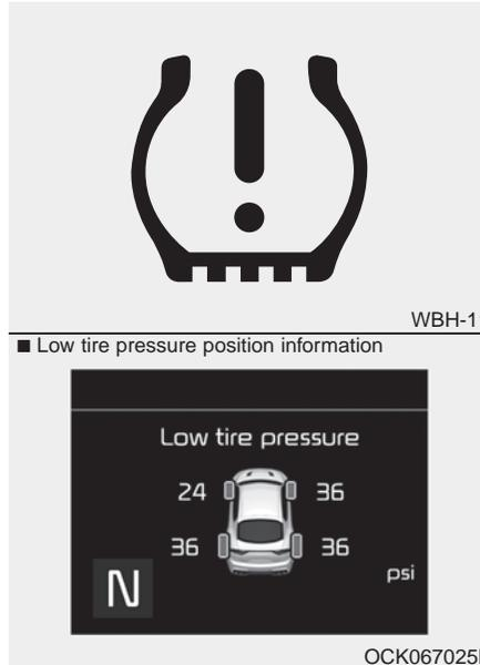
When the tire pressure monitoring system warning indicators are illuminated, one or more of your tires is significantly under-inflated.
