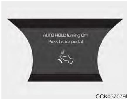
When the conversion from Auto Hold to EPB is not working properly a warning will sound and a message will appear.
