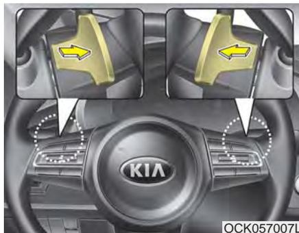
The paddle shifter is available when the shift lever is in the D (Drive) position.
