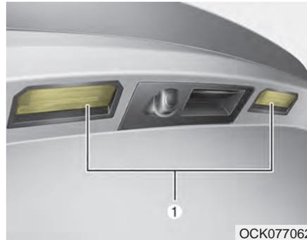
If the license plate lamp (LED) (1) does not operate, have the vehicle checked by an authorized Kia dealer. The LED lamps cannot be replaced as a single component because they are part of an integrated unit. The LED lamps have to be replaced with the unit.
