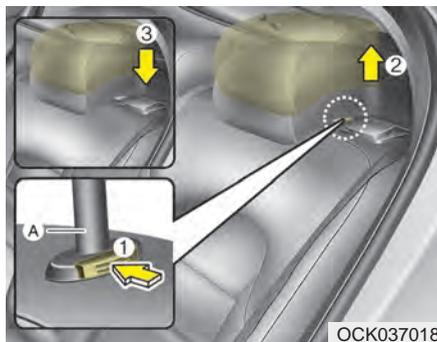
**Removal and reinstallation (if equipped)**
