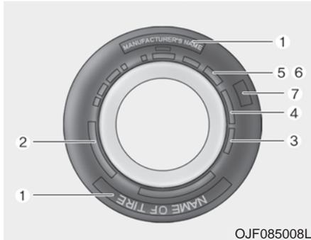
This information identifies and describes the fundamental characteristics of the tire and also provides the tire identification number (TIN) for safety standard certification. The TIN can be used to identify the tire in case of a recall.
