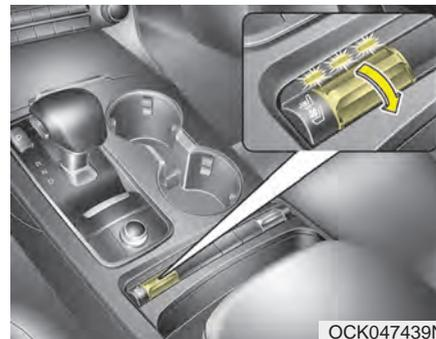
The temperature setting of the seat changes according to the switch position.
