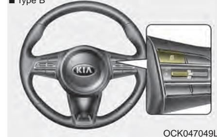
The LCD display modes can be changed by using the control buttons on the steering wheel.
