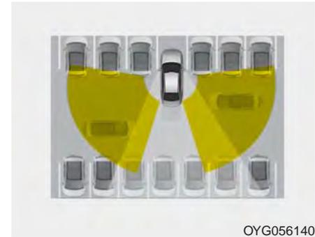
When your vehicle moves backwards from a parking position, the sensor detects approaching vehicles to the left or right side direction and gives information to the driver.
