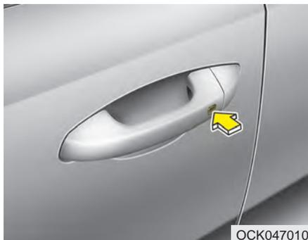
Pressing the button of the front outside door handles with all doors closed and any door unlocked, locks all the doors. The hazard warning lights will blink and the chime will sound once to indicate that all doors are locked. The button will only operate when the smart key is within 28~40 in. (0.7~1 m) from the outside door handle. If you want to make sure that a door has locked or not, you should check the door lock button inside the vehicle or pull the outside door handle.
