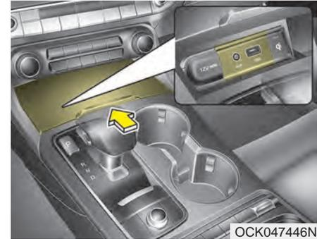
You can use an AUX port to connect audio devices and a USB port to plug in a USB or iPod®.
