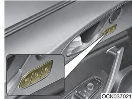
Driver Position Memory System is the facility that enables driver's seat, leg extension, steering wheel, exterior mirrors, cluster and head-up display (HUD) to be controlled with a simple button operation, which allows a driver to recall memorized driving positions and automatically control them.
