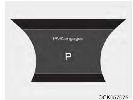
The message appears on the LCD display, when the P (Park) position is engaged.
