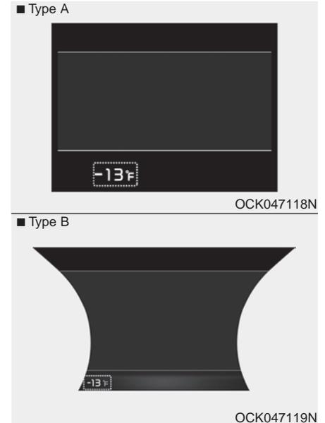
This gauge indicates the current outside air temperatures by 1°F (1°C).
