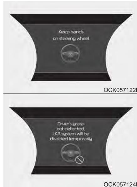
If the driver takes hands off the steering wheel for several seconds while the LKA is activated, the system will warn the driver.
