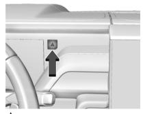
A: Press this button to make the front and rear turn signal lamps flash on and off. Press again to turn the flashers off. When the hazard warning flashers are on, the vehicle turn signals will not work.
