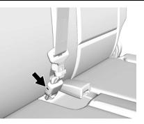
4. Disconnect the rear seat belt mini-latch, using a key in the slot on the mini-buckle, and let the belt retract into the headliner.
