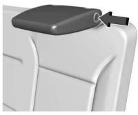
The head restraint will fold forward automatically.
