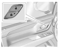
**G** : Press to lock the doors. The indicator light in the switch will illuminate when locked.
