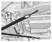
The vehicle is equipped with specific attachment points to be used to pull the vehicle onto a flatbed car carrier from a flat road surface. Do not use these attachment points to pull the vehicle from snow, mud, or sand.
