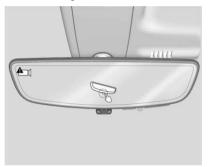
See your dealer for service if a blue screen and are displayed in the mirror, and the display shuts off. Also, push the tab as indicated to return to the automatic dimming mode.
