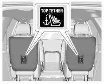
For non-executive seats, the top tether anchors are on the rear of the seatback for each seating position in the second row. Be sure to use an anchor located directly behind the seating position where the child restraint will be placed.
