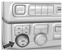
Turn the knob left or right to select the desired ride height in the menu. To finalize the selection, either press the Ride Height button again or wait three seconds for the menu to timeout. Ride Heights that are unavailable are greyed out in the menu.
