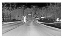
With the Front Pedestrian Braking system turned on, Night Vision provides a red Head-Up Display (HUD) alert, if equipped, when the system detects that the vehicle is approaching a pedestrian or large animal ahead too quickly. In addition, an alert beeps or the Safety Alert Seat pulses, if equipped. See Front Pedestrian Braking (FPB) System ▷ 267.
