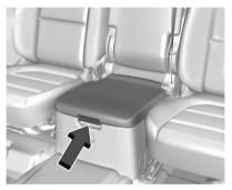
If equipped, you can lock the front center seat storage with the mechanical key inside the remote key. See *Keys*  $\Rightarrow$  7.
