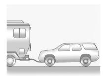
Only dinghy tow four-wheel-drive vehicles with a two speed transfer case that has an N (Neutral) and a  $4\downarrow$  setting.
