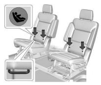
For non-executive seats, the lower anchors are located in the crease between the seatback and seat cushion.
