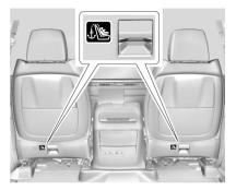
Executive seating top tether anchors are on the lower structure of seat back behind a fabric slit. Slide the seat forward to access the anchor. Be sure to use an anchor located directly behind the seating position where the child restraint will be placed. See Second Row Seats  $\Rightarrow$  45.
