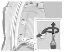
4. Remove the flat tire secure strap from the glove box and place the loop end of the strap through the cargo tie-down. Place the
