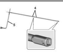
2. Assemble the jack handle extensions (4) and wheel wrench (5), as shown.
