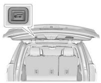
Press any liftgate button, the touch pad, or  $\overline{\mathscr{L}}$ on the remote key while the liftgate is moving to stop it. Pressing any liftgate button or pressing  $\overline{\mathscr{L}}$  twice quickly on the remote key restarts the operation in the reverse direction. Pressing the touch pad on the liftgate handle will restart the motion, but only in the opening direction.
