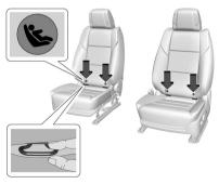
Executive seating lower anchors are in the crease between the seatback and the seat cushion. Push the seatback trim up at the crease to access the lower anchor.
