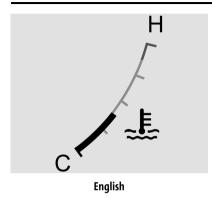
This gauge shows the engine coolant temperature.
