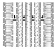
Treadwear indicators are one way to tell when it is time for new tires. Treadwear indicators appear when the tires have only 1.6 mm (1/16 in) or less of tread remaining. See *Tire Inspection*  $\Rightarrow$  362 and *Tire Rotation*  $\Rightarrow$  362.
