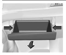
2. Press the sides of the glove box bin inward to clear the stoppers and rotate downward to lower the bin.
