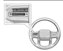
S: Press to turn cruise control on or off. When ACC is the selected cruise control mode, the ACC light - is lit white on the instrument cluster. +RES : Press the thumbwheel up briefly to resume the previous set speed or use to increase vehicle speed if ACC is already activated. To increase speed by about 1 km/h (1 mph), briefly press the thumbwheel up to +RES and release it. To increase speed to the next 5 km/h (5 mph) mark on the speedometer, press up to +RES and hold.
