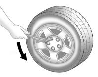
Use the wheel wrench to loosen all the wheel nuts. Turn the wheel wrench counterclockwise to loosen the wheel nuts. Do not remove the wheel nuts yet.
