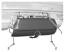
To remove hitch cover, if equipped:
