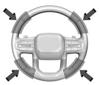
To begin steering manually, hold the steering wheel firmly with both hands using the highlighted regions. The Super Cruise light will display red and a message will display in the DIC. In addition, beeps will sound, or the Safety Alert Seat will vibrate, if equipped. To view collision and detection settings from the infotainment home screen, touch Settings > Vehicle > Collision/Detection Systems. When you begin steering manually, Super Cruise will disengage.
