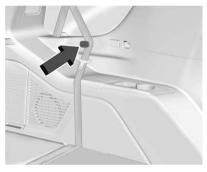
6. Stow the seat belt in the belt stowage clip. Repeat the steps to fold the other seatback, if desired.
