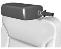
The head restraint will fold forward automatically.
