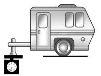
The Maximum Trailer Tongue Weight Rating for a conventional trailer hitch is shown on the Trailering Information Label.
