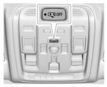
There are dome lamps in the overhead console. The dome lamps come on when any door is opened, a on the remote key is pressed, or when the vehicle is turned off.
