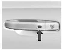
The remote key must be within 1 m (3 ft) of the liftgate or door being opened or locked. Press the button on the door handle to open. See "Keyless Access Operation" in *Remote Key Operation* rightarrow 8.
