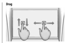
Drag is used to move applications on the infotainment home screen, or to pan the map. To drag the item, it must be held and moved along the display to the new location. This can be done up, down, right, or left. This feature is only available when vehicle is parked and not in motion.
