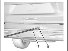
Insert the hoist end (open end) of the extension tool (7) through the hoist shaft access hole (8) in the rear bumper until you feel engagement with the hoist assembly (1). Only a minimal amount of the jack handle extension end will be visible.
