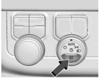
If equipped, the button for the front fog lamps is on the exterior lamp control, to the left of the steering column.
