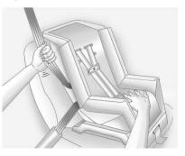
To tighten the belt, push down on the child restraint, pull the shoulder portion of the belt to tighten the lap portion of the belt, and feed the shoulder belt back into the retractor.
