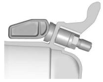
Contact your trailer service center or tire service center to have the pressure sensors installed inside the trailer tires. The technician should insert the sensor stem through the hole in the trailer wheel. When the sensor is correctly positioned, the nut on the sensor stem should be tightened to  $8 N \cdot m(6 \ lb \ ft)$ . When mounting the trailer tire onto the trailer wheel be careful not to damage the sensor.
