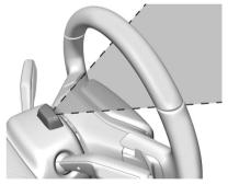
Sunglasses, hats, or other types of clothing that change the shape of the head may interfere with camera performance. To improve camera performance, raise or lower the steering wheel, or change the seat position. Driver Attention Assist does not record video or audio. It is only active while driving with the feature enabled.
