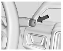
**P:** This position locks the drive wheels. Use P (Park) when starting the vehicle to ensure the vehicle does not move.
