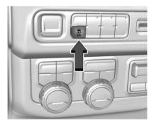
The button for the Traction Control System and the StabiliTrak/Electronic Stability Control system is on the instrument panel to the left of the steering wheel.
