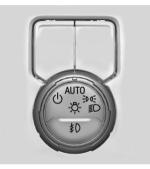
The exterior lamp controls are on the instrument panel to the left of the steering wheel.
