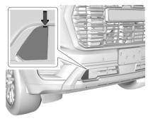
3. Remove the engine heater connector cover by gently prying the small notch with a flat blade tool.
