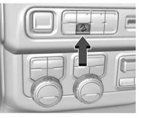
Press <sup>2</sup>/<sub>4</sub> to enable or disable HDC. Vehicle speed must be below 60 km/h (37 mph).
