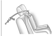
2.3 If the position you are using has a fixed headrest or head restraint and you are using a single tether, route the tether around the inboard or outboard side of the headrest or head restraint.
