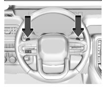
ERS, or Manual Mode, allows for the selection of the range of gear positions. Use this mode when driving downhill or towing a trailer to limit the top gear and vehicle speed. The shift position indicator within the Driver Information Center (DIC) will display a number next to the L indicating the highest available gear.
