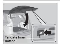
Press the tailgate inner button on the tailgate to close the power tailgate.
