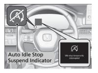
The Auto Idle Stop suspend indicator comes on and a message appears on the gauge when the Auto Idle Stop system cannot be activated.
