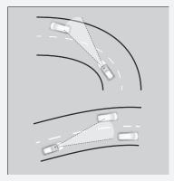
When the vehicle ahead of you moves away, such as when entering an interchange or rest area, ACC with Low Speed Follow may continue to maintain the set following-interval for a short time.
