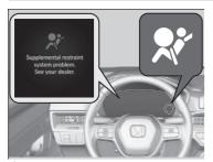
■ When the power mode is set to ON The indicator comes on for a few seconds, then goes off. This tells you the system is working properly.
