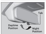
Flip the tab to switch the position.
