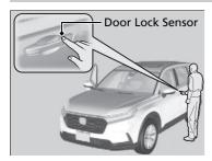
The vehicle will automatically lock after you lock the doors in advance then close the doors and tailgate.
