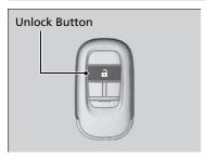
**To open:** Press the unlock button, and then within 10 seconds, press it again and hold it. If the windows stop midway, repeat the procedure.
