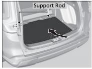
**4.** Push the far end of the floor lid down to the bottom under the support rods, then lower the other end.
