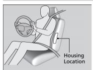
The side airbags are housed in the outside edge of the driver's, passenger's, and rear outer passenger's seat-backs.
