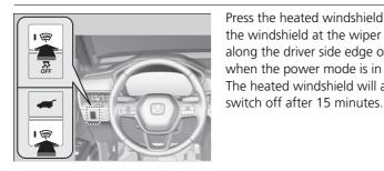
Press the heated windshield button to deice the windshield at the wiper park area and along the driver side edge of the windshield when the power mode is in ON. The heated windshield will automatically
