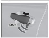
Pull and hold the outer handle. Insert the key into the key cylinder completely from below the handle.
