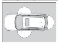
When you carry the keyless remote, you can lock/unlock the doors, tailgate, and fuel fill door.
