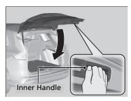
When all the doors are unlocked or you press the tailgate unlock button\* on the remote transmitter, the tailgate is unlocked. Press the tailgate outer handle and lift open the tailgate.
