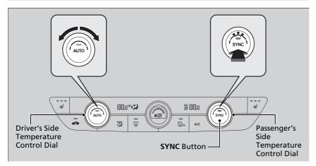
You can set the temperature synchronously for the driver's side and the passenger's side in synchronization mode.
