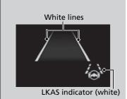
When the LKAS is suspended, green lines on the gauge change to white lines or disappear, and the beeper sounds (if activated).
