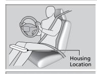
Housing Location The knee airbag for the driver and the one for the front passenger are housed under the steering column and the glove box respectively.
