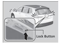
Touch the door lock sensor on the front door or press the lock button on the tailgate.
