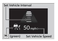
When ACC with Low Speed Follow starts operating, the vehicle icon, interval bars and set speed appear on the gauge.
