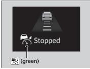
Your vehicle also stops, automatically. The **Stopped** message appears on the gauge. When the vehicle ahead of you starts again, if you press the **RES/+/SET/-** switch up or down, or depress the accelerator pedal, ACC with Low Speed Follow will operate again within the prior set speed.
