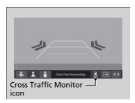
The system can be turned on and off on the audio/information screen by pressing the Cross Traffic Monitor icon.
