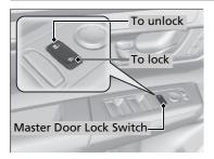
Press the master door lock switch in as shown to lock or unlock all doors, tailgate, and fuel fill door.
