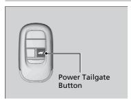
Press the power tailgate button for more than one second to operate when the power mode is in VEHICLE OFF.
