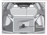
The cargo hooks on the both of the cargo area can be used to hang a light items.
