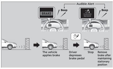
If the only rear sensors are turned off using the parking sensor system, the assistive braking will not work when reversing.
