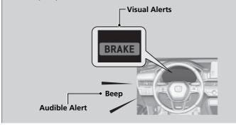
You can change the distance (**Long/Normal/Short**) between vehicles at which the system's earliest collision alert will come on.
