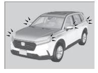
If the engine starts successfully, some exterior lights flash six times.
