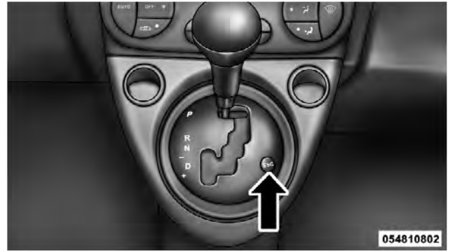
ESC Off Switch (Automatic Transmission)
