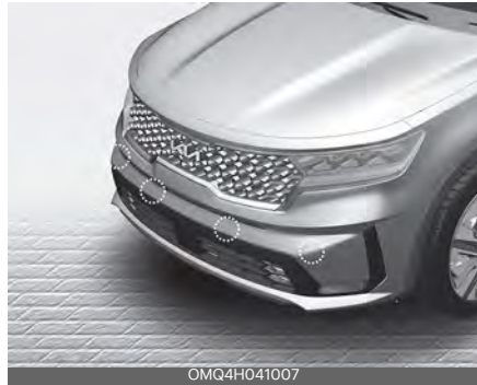
Front corner ultrasonic sensors
