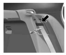
Place the outboard seat belt in the seat belt clip on the side trim of the vehicle.
