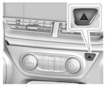
Press the  $\triangle$  button to make the front and rear turn signal lights flash on and off. This warns others that you are having trouble. Press again to turn the flashers off.
