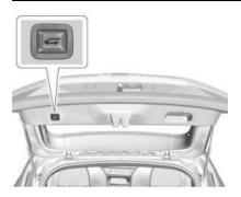
Press any liftgate button, the touch pad, or  $\cancel{S}$ on the remote key while the liftgate is moving to stop it. Pressing any liftgate button or pressing  $\cancel{S}$  twice quickly on the remote key restarts the operation in the reverse direction. Pressing the touch pad on the liftgate handle will restart the motion, but only in the opening direction
