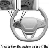
☺ : Press to turn the system on or off. The indicator turns white on the instrument cluster when ACC is turned on.
