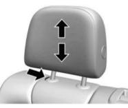
To lower the head restraint, press the button on the top of the seatback and push the head restraint down. After releasing the button, ensure the head restraint locks in place and is unable to move up or down.
