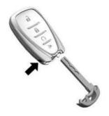
To remove the key, press the button on the side of the remote key and pull the key out. Never pull the key out without pressing the button. If it becomes difficult to turn the key, inspect
