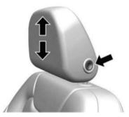
The height of the head restraint can be adjusted.
