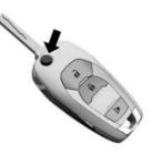
Press the key release button on the remote key to extend the key blade. Press the button and the key blade to retract the key.
