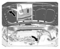
3. Lift the hood and release the hood prop from its retainer, above the radiator. Securely place the hood prop into the slot on the underside of the hood.
