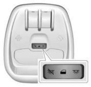
Dome lights provide overhead interior lighting. The dome light switch is in the overhead console and has three positions.
