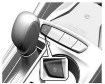
The automatic engine stop/start feature can be disabled and enabled by pressing  ${}^{(A)}_{\text{DFF}}$ . Auto Stop is enabled each time you start the vehicle.
