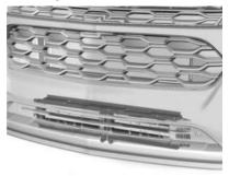
This vehicle may have a shutter system that automatically closes the frontal cooling opening. This system is designed to help improve fuel economy. Ensure the shutter system is clear of any visible debris, snow, or ice. If the Malfunction Indicator Light activates and remains lit after clearing the shutter system, see *Malfunction Indicator Light (Check Engine Light)* \$ 95.
