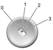
0. Stopping the Engine/LOCK/OFF
