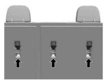
For models with a cargo cover, the top tether anchors are on the back of the rear seatbacks. Remove the cargo cover before installing the top tether. The cargo cover should remain off while the top tether is in use. Be sure to use an anchor directly behind the seating position where the child restraint will be placed.
