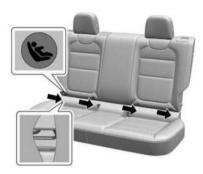
The outboard lower anchors are behind the vertical openings in the seat trim.
