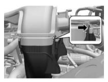
2. Disassemble the duct.
