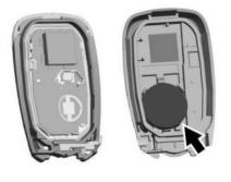
3. Remove the battery by pushing on the battery and sliding it toward the bottom of the remote key.
