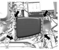
3. Remove four screws, tilt the cover, and slide it out of the assembly.
