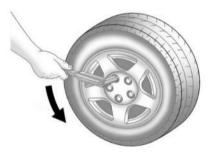
2. Turn the wheel wrench counterclockwise to loosen the wheel nuts. Do not remove them yet.
