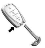
1. Press the button on the side of the remote key to remove the key. Never pull the key out without pressing the button.
