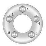
13. Tighten the wheel nuts firmly with the wheel wrench in a crisscross sequence, as shown.
