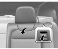
1. Pull the lever on top of the seatback to unlock the seatback.
