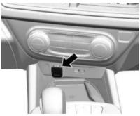
Certain accessory plugs may not be compatible with the accessory power outlet and could overload vehicle and adapter fuses. If a problem is experienced, see your dealer. When adding electrical equipment, be sure to follow the proper installation instructions included with the equipment. See Add-On Electrical Equipment ⇔ 220.
