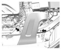
1. Remove the two push pins.
