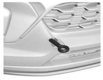
Install the tow eye into the socket and turn it until it is fully tightened. When the tow eye is removed, reinstall the cover with the notch in the original position.
