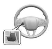
**(***i*): If equipped with a heated steering wheel, press to turn on or off. A light near the button displays when the feature is turned on.
