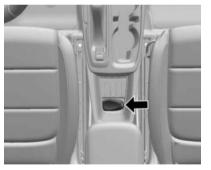
1. Place the remote key in remote key pocket with the buttons facing the front of the vehicle.
