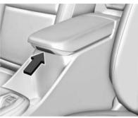
There is storage under the armrest in the center console. Press the button and lift to open.
