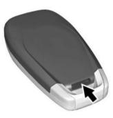
1. Separate the two halves of the remote key by inserting a flat tool into the recess of the remote key.
