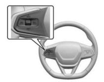
$\mathfrak{S}$ : Press to turn cruise control on and off. The white cruise control indicator light comes on in the instrument cluster when cruise control is turned on.
