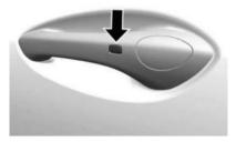
The remote key must be within 1 m (3 ft) of the liftgate or door being opened. Press the button on the door handle to open. See *Remote Key Operation (Keyless Access)*  $\Rightarrow$  10 *Remote Key Operation (Key Access)*  $\Rightarrow$  15.
