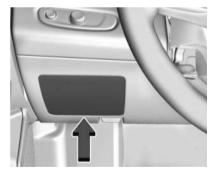
The instrument panel fuse block is on the underside of the driver side instrument panel. To access the fuses, remove the storage compartment. To remove the storage compartment, open the compartment and pull it out.
