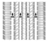
Treadwear indicators are one way to tell when it is time for new tires. Treadwear indicators appear when the tires have only 1.6 mm (1/16 in) or less of tread remaining. See *Tire Inspection*  $\Rightarrow$  264 and *Tire Rotation*  $\Rightarrow$  264.
