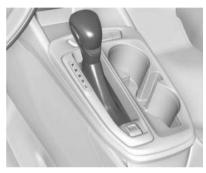
**P**: Use P (Park) when starting the engine because the vehicle cannot move easily. This position locks the front wheels.
