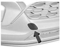
Carefully open the cover on the fascia by using the small notch that conceals the tow eye socket.
