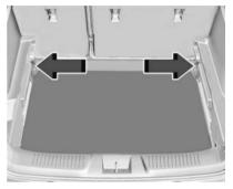
The cargo management system has an angle adjustment to secure the load floor while removing stored items.
