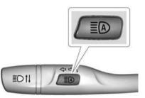
To enable the IntelliBeam system, turn the headlight control to either AUTO or D, then press  $\fbox{A}$  on the turn signal lever.
