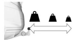
The permissible gross weight of the loaded rear carrier depends on how far its center of gravity is from the ball head.
