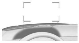
Head-up display views are projected onto the windshield through a protective glass. The protective glass is located between the steering wheel and windshield.
