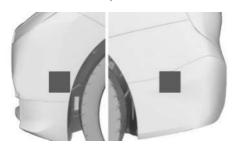
The ultrasonic sensors for the parking assistance systems are located on the sides of the front and rear bumpers.
