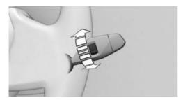
Turn the thumbwheel on the wiper lever.
