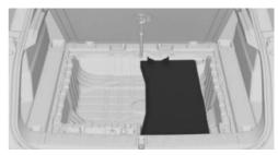
The cargo cover can be stowed under the cargo area floor.
