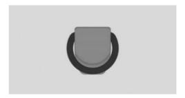
The lashing eyes are located in the cargo area. The front lashing eyes are located under covers.
