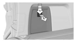
2. If necessary, remove the cargo cover from the storage under the cargo area floor. Cargo cover, refer to page 312.
