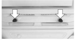
Setting the air flow direction and air volume at the vent.
