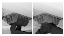
3. Extend the jack by turning the jack crank handle or lever clockwise.
