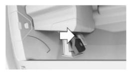
Slide the fragrance cartridge into the cartridge holder at a slight angle without applying pressure. The fragrance cartridge is correctly positioned when the cartridge holder can be closed.
