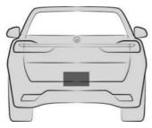
The Rear View Camera is located above the license-plate carrier.
