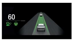
An example of active Driver Assistance: Indicator and warning lights for Distance Control and Assisted Driving Mode are displayed. At the same time, the Distance Control is animated in Assisted View.
