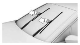
3. Press the button, arrow 1, turn the wiper blade slightly clockwise, and pull it forward and out, arrow 2.
