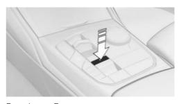
Press button P. The transmission lock is engaged.
