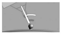
Two static circular segments help to estimate the distance of the trailer to the trailer hitch.
