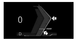
Needle in range of arrow 1: display for energy recovery such as while decelerating CHARGE. Needle in range of arrow 2: the drive power in percent, POWER.
