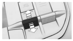
Repeatedly push the rocker switch forward or pull it back until the desired xOFFROAD driving mode is displayed on the instrument cluster.
