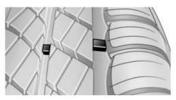
The tire manufacturer's wear indicators are distributed around the tire circumference and have a height of at least 0.06 in/1.6 mm.
