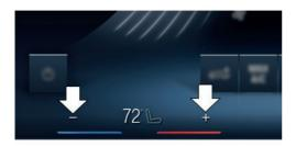
You can set the desired temperature for driver and front passenger individually on the menu har.
