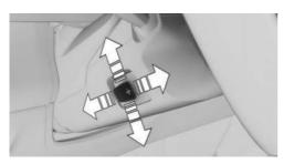
Press the switch to adjust the steering wheel forward/back position and height to the seat position.
