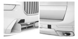
The towing eye thread is located behind a cover on the front and rear bumper.
