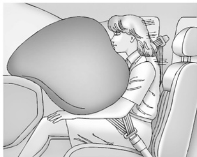
The front outboard passenger frontal airbag is in the passenger side instrument panel.
