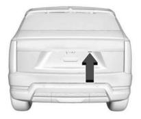
If equipped, press the button above the license plate to open the liftglass, or press twice quickly on the remote key. Do not leave the liftglass open when raising the liftgate.
