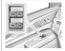
The power windows work when the vehicle is on.
