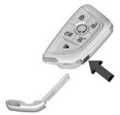
Press the button on the side of the remote key near the bottom and pull the mechanical key out. Never pull the mechanical key out without pressing the button.
