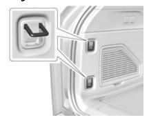
There are four cargo tie-downs in the rear cargo area and four in the underhood compartment, which can be used to secure cargo and keep it from moving inside the vehicle.
