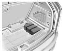
Release the straps securing the tire sealant and compressor kit, then remove the kit.
