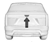
To open the liftgate, press on the power door lock switch or press on the remote key twice to unlock all doors, then press the emblem.
