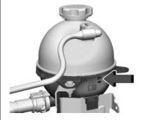
If the coolant level is not visible or needs to be adjusted within the reservoir, contact your dealer.
