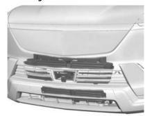
The vehicle may have a shutter system that automatically closes the frontal cooling openings. This system promotes airflow around the vehicle, reducing drag and providing energy savings. Ensure the shutter system is clear of any visible debris, snow, or ice. If the Service Vehicle Soon light activates and remains after clearing the shutter system, see Service Vehicle Soon Light
