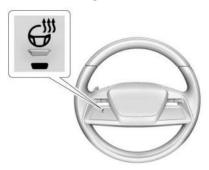
: Press to turn the heated steering wheel on or off. An indicator next to the button is lit when the feature is turned on.
