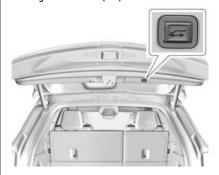
Press on the bottom edge of the liftgate next to the latch to close.
