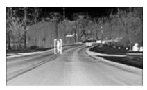
With the Front Pedestrian Braking system turned on, Night Vision provides a red Head-Up Display (HUD) alert, if equipped, when the system detects that the vehicle is approaching a pedestrian or large animal ahead too quickly. In addition, an alert beeps or the Safety Alert Seat pulses, if equipped. See Front Pedestrian Braking (FPB) System ▷ 260.
