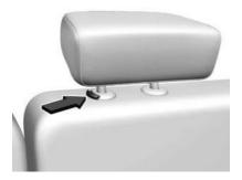
Pull the head restraint up to raise it. Try to move the head restraint to make sure that it is locked in place.
