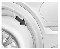
Pull the emergency manual charge cord release handle. The DC charge cord will release.
