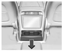
If equipped, there may be two cupholders, two USB ports, two HDMI ports, and a power outlet on the back of the center console. To access the cupholders, press and release the cover.
