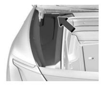
The Underhood Compartment Fuse Block is under a cover and side extension/shield in the underhood compartment. Remove the shield, starting at the top. Once the shields clips disengage, the tabs along the bottom can disengage to remove the left side access cover.
