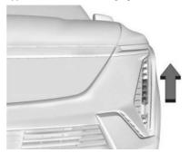
The headlight Charge Status Indicator bar is located on the headlights. As charging occurs, the blue light bars on the headlights fill towards the top of the vehicle.
