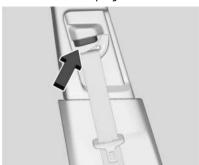
Push the release button to move the height adjuster to the desired position.
