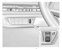
Rotate this thumbwheel  $\mathcal{E}^{\mathfrak{F}}$  to adjust the brightness of all illuminated controls. The thumbwheel is on the instrument panel to the left of the steering wheel.
