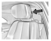
Executive second row seats have adjustable head restraints. To raise/lower the head restraint/headrest, press the button located on the side of the head restraint, and push the
