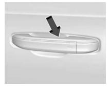
To unlock and open any door, squeeze the switch on the inside grip area of the outside door handle.
