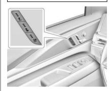
The manual buttons are located on the door panel. To operate, the vehicle must be on.
