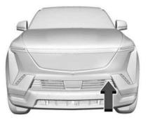
To open or close the hood, press the touchpad on the front fascia once. The remote key must also be within 1 m (3 ft) if the vehicle is locked. To stop the hood while in motion, press the touchpad.
