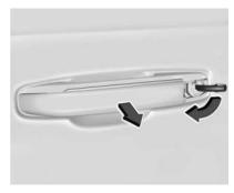
4. Insert the mechanical key in the cylinder.
