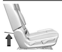
Pull the strap on the bottom rear of the second row seat to release the seatback. The seatback will fold forward.
