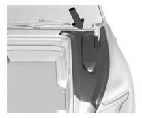
The coolant reservoir is under a cover and side extension/shield in the underhood compartment. Unclip the right side of the shield and remove the right side access cover.
