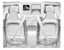
Executive seating top tether anchors are on the lower structure of seat back behind a fabric slit. Slide the seat forward to access the anchor. Be sure to use an anchor located directly behind the seating position where the child restraint will be placed. See Second Row Seats \$\displays\$ 50.
