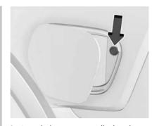
3. Press the button to manually close the charge port door.
