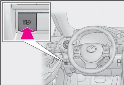
Press the Automatic High Beam switch.
