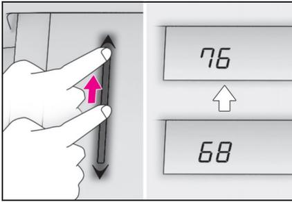
To adjust the temperature setting, touch and slide your finger up or down on the sensor.
