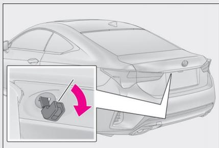
Turn the mechanical key clockwise to open.
