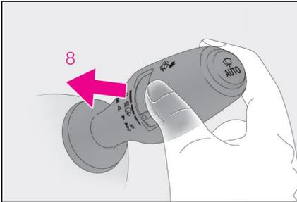
When AUTO mode is selected, the sensor sensitivity can be adjusted by turning the switch ring.
