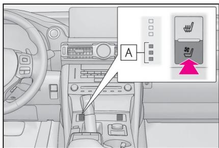
Each time the switch is pressed, the intensity of the seat ventilator changes and the level indicator lights (green) **A** light as follows:
