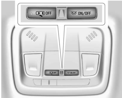
Dome Lamp Controls
