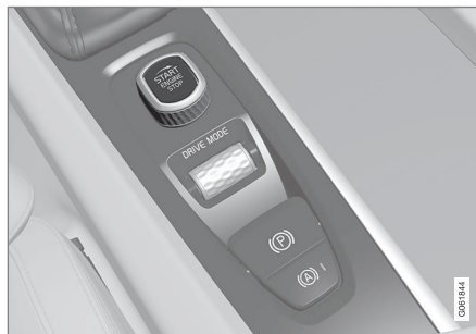
Start knob in the tunnel console.
