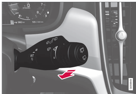
Washing function, right-hand steering wheel lever.
