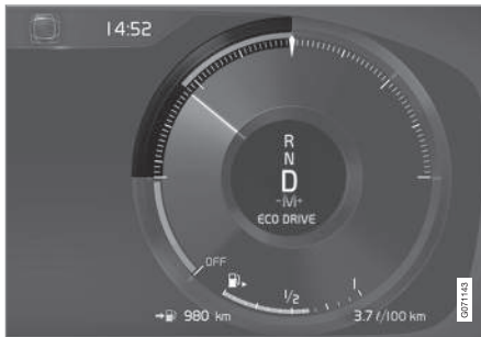
Eco gauge in 12" instrument panel*.
