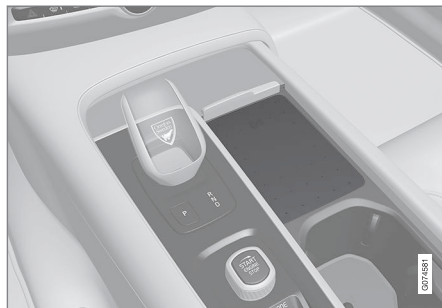
Wireless phone charger in the tunnel console.
