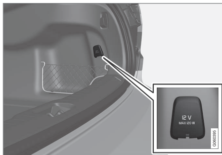
12 V outlet in trunk/cargo compartment*.
