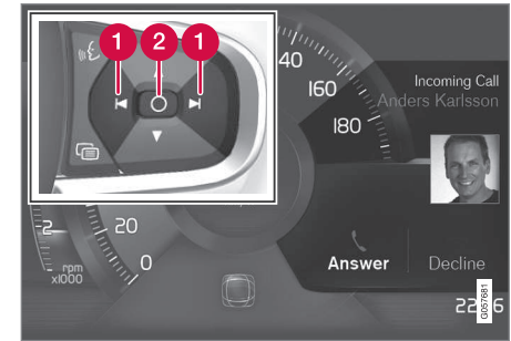
Examples of messages in the instrument panel 4 and the right-side steering wheel keypad.
