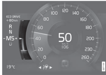
Eco gauge in 8" instrument panel.
