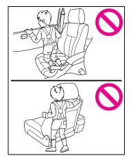
In the event of an accident, the force of SRS side airbag and/or SRS curtain shield airbag deployment could injure the child seriously because his/her head, arms or other parts of the body are too close to the SRS side airbag and/or SRS curtain shield airbag.
