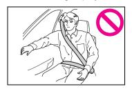
Do not place any objects over or near the SRS airbag cover or between you and the SRS airbag. If the SRS airbag deploys, these objects could interfere with its proper operation and could be propelled inside the vehicle, causing injury.
