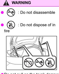
Do not pull on the trunk damper stay to close the trunk, and do not hang on the trunk damper stay.
